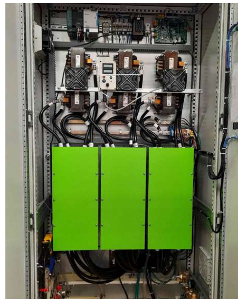
Level 3+ ultrafast EV charger example using 3 x HIPO400AT6
