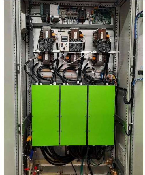
Level 3+ ultrafast EV charger example using 3 x HIPO400AT6
