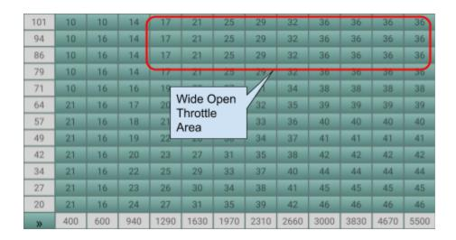
**6. High RPM/Low load**- This area of the table is not used much unless the driver is purposely holding the car in a low gear at high RPM with light throttle. Timing should be very high around 40-50 degrees. Retarding timing here will excessively heat exhaust components.
