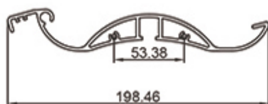
model: 19827 wall thickness: 2mm single weight: 5.35kg/m
