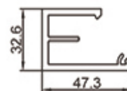
model: XT4732 wall thickness: 3.3mm single weight: 1.04kg/m
