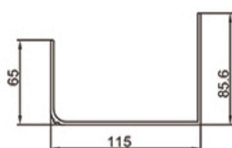
model: GL115*85 wall thickness: 2.2mm single weight: 1.55kg/m
