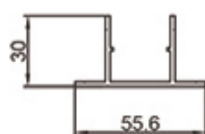
model: CL5530 wall thickness: 2.0mm single weight: 0.61kg/m
