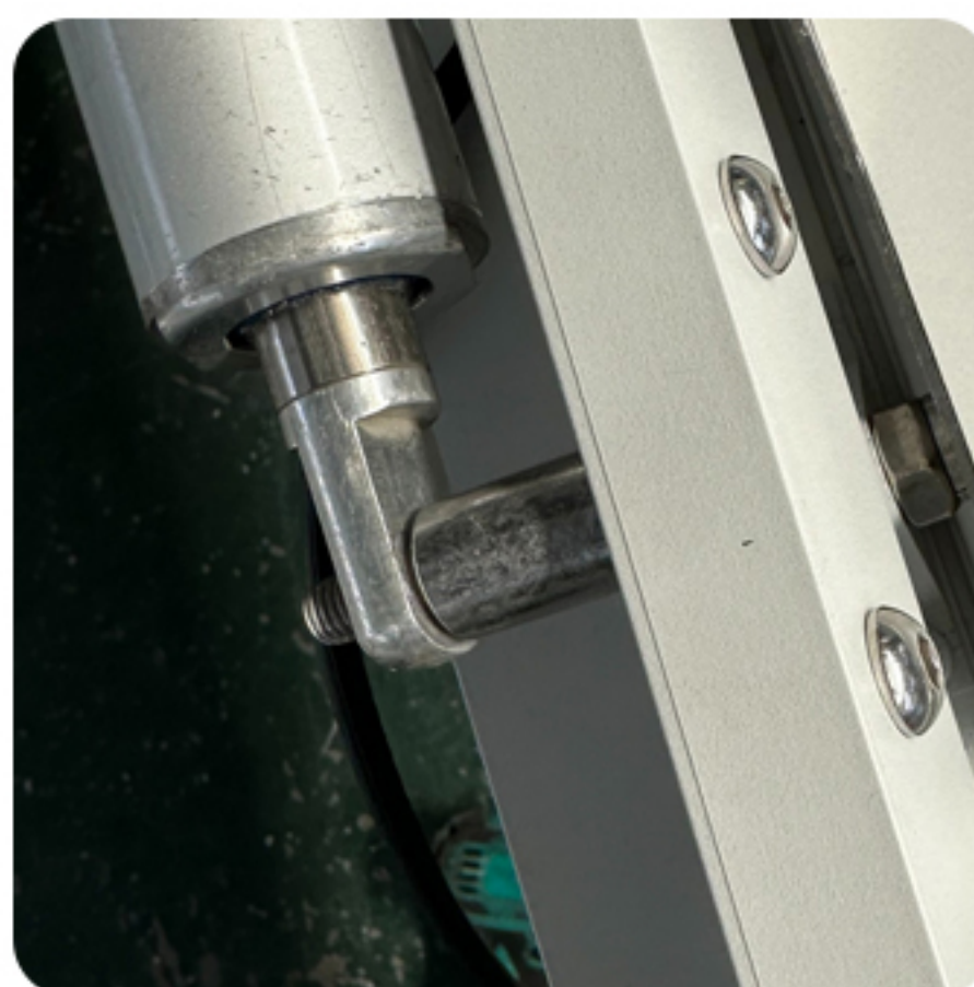
Fix the motor, thread the bolts, and tighten the screws (1 washer facing inward and 2 washers facing outward)
