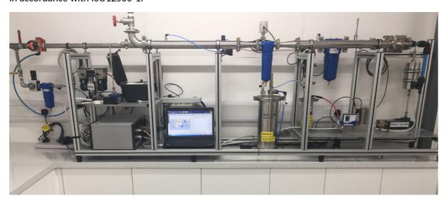
As a result, all elements manufactured by KSI Technologies have now had their oil classes validated according to ISO8573-1 self-certified in accordance with ISO12500-1. Furthermore, through extensive research and development KSI Technologies can offer some of the lowest pressure drops on the market.
