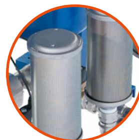
Large-dimensioned silencers on all ATK models
