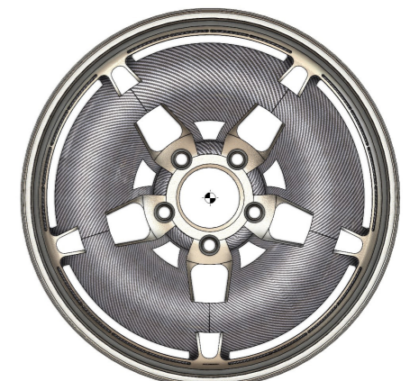
Fig. 59. CB1 and CSP2 Assembled, showing centre of mass
