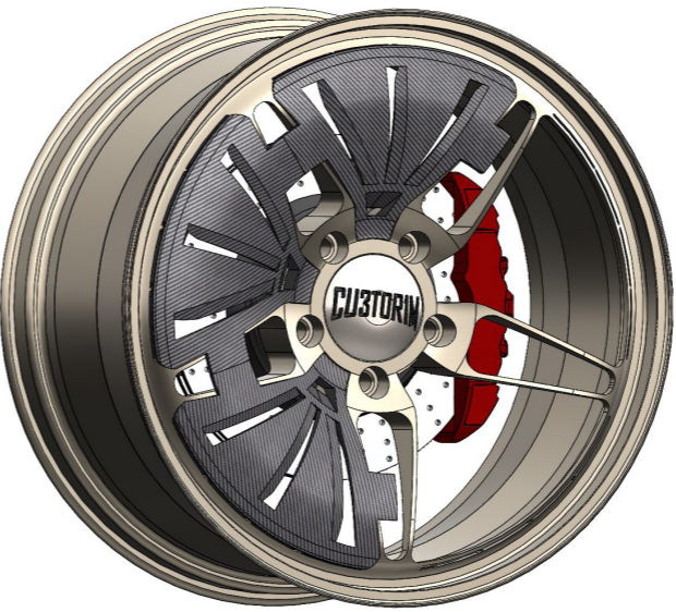
Fig. 63. Brake disc and caliper assembled on to the CB1+ CSP1
