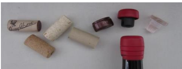
Wine closures from left: Natural cork, Agglomerate, 1+1, Synthetic, Screw Cap, Zork, Vinolok
