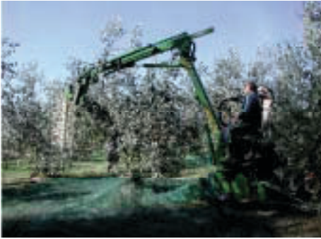
Figure 19. Reel-type beater with radial rods.
