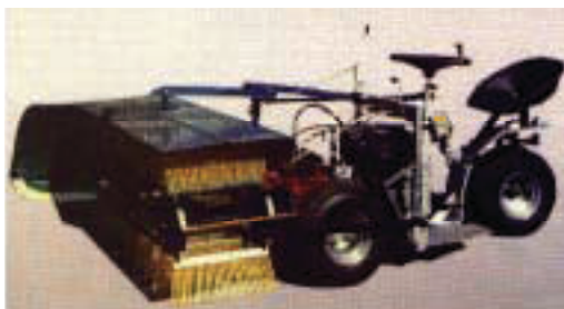
Figure 38. Windrower for olives harvested from the ground.
