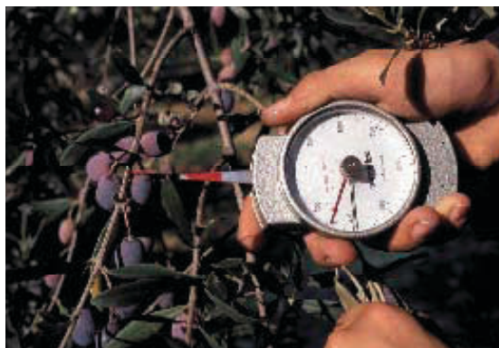
Figure 5. Dynamometer with spiked sensor for determining fruit removal force.
