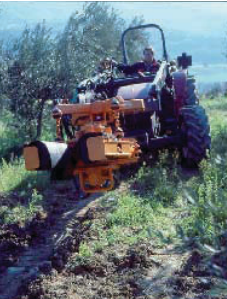
Figure 21. Shaker with two vibrating masses and two engines.
