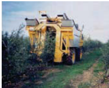
Figure 25. Shaker featuring larger shaker cage.
