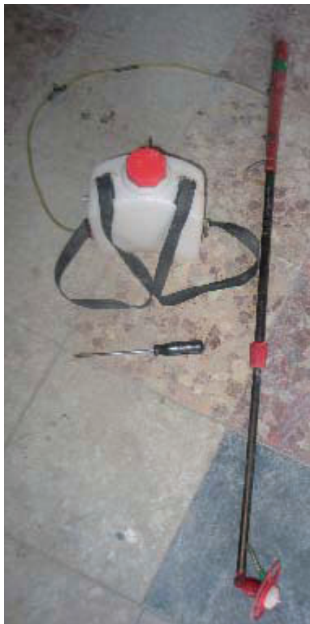
Figure 3. Battery-operated sprayer with centrifugal spray tip.
