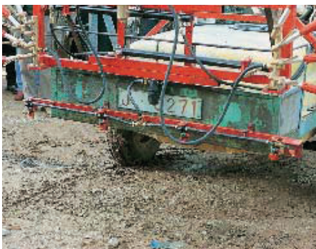
Figure 4. Power-driven sprayer with large-capacity tank and front and rear booms.
