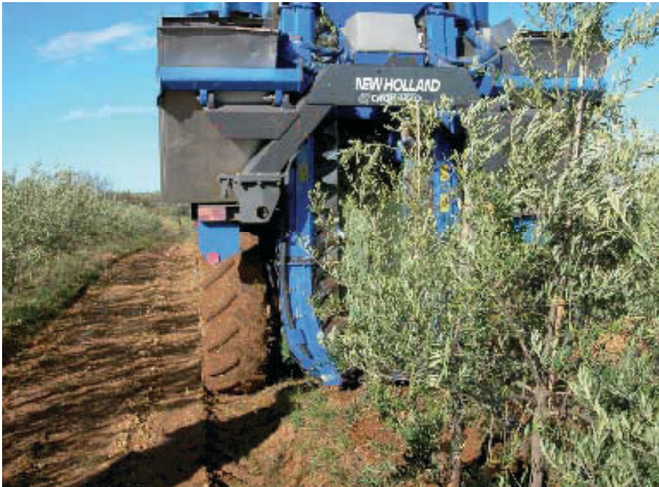
Figure 31. Superintensive orchard with over-the-row harvester.
