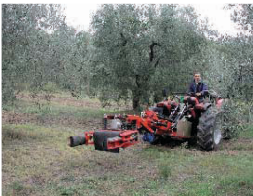
Figure 23. Shaker with a single eccentric mass.
