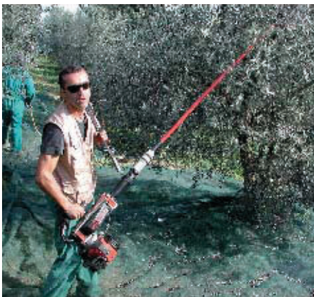
Figure 17. Mechanical hand-carried shaker.
