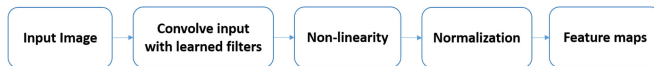
Fig. 3. Feature Extraction Using Convolutional Neural Networks (CNNs): Convolutional operation is performed by moving the filters with fixed stride through the input image and computing the convolution between each filter matrix and input image matrix. Non-linearity is introduced after each convolutional operation by applying a Rectified Linear Unit (ReLU) since convolution is a linear operator. Features are extracted from the fully connected layer right before the classification layer.
