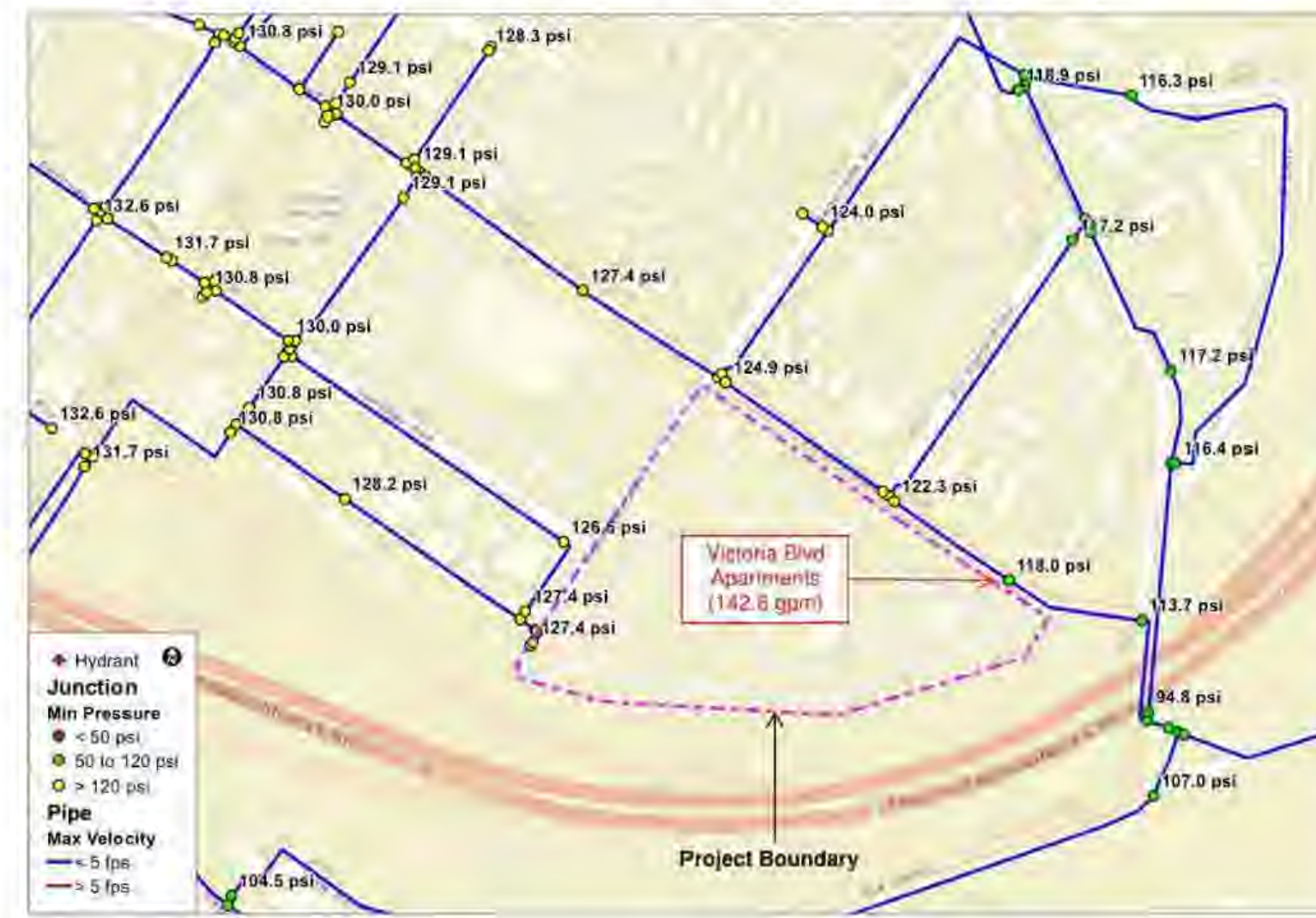
Figure 2-1: Existing (2020) MDD with Victoria Blvd Apartments MDD Analysis Results - Minimum Pressures and Maximum Velocities
