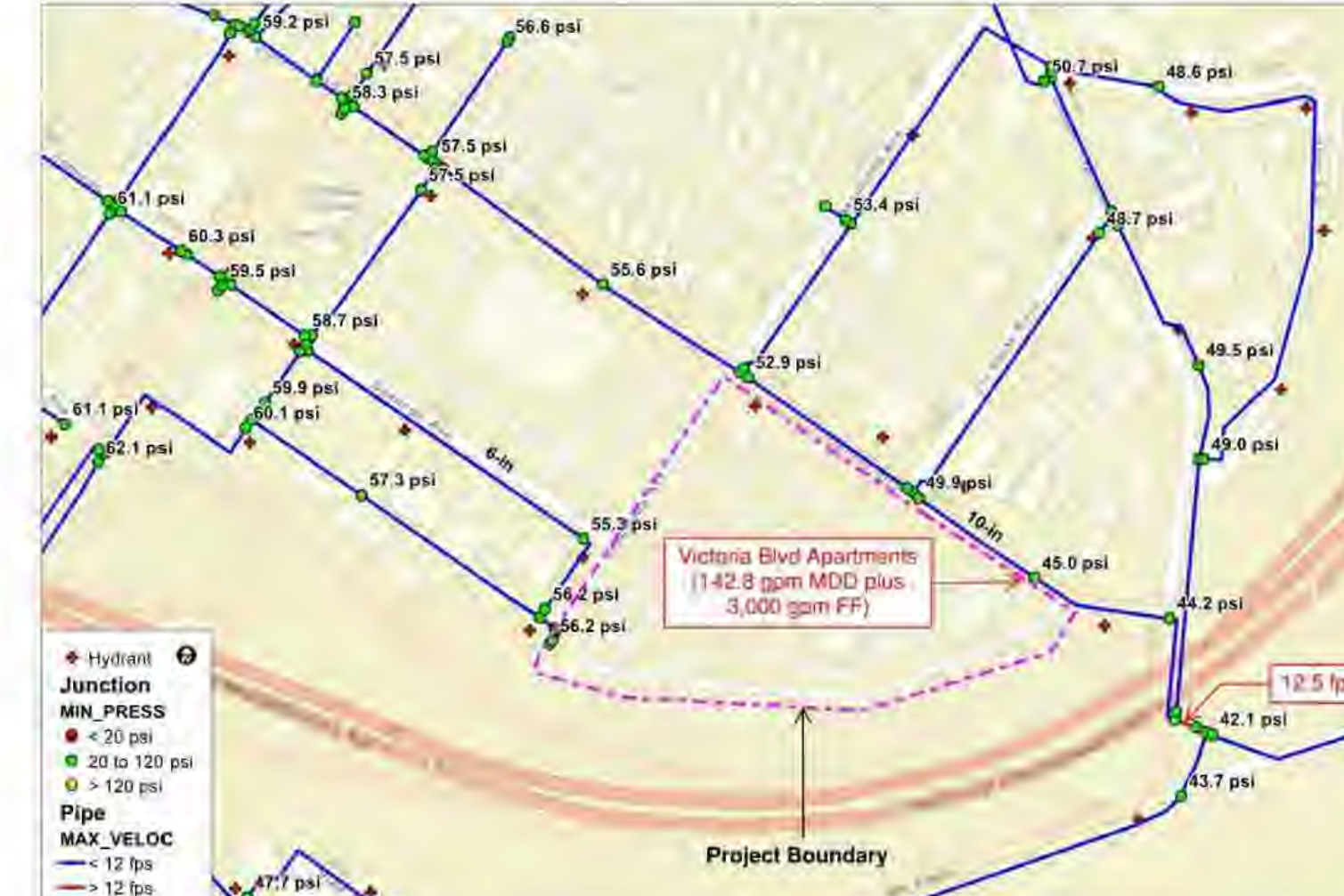
Figure 2-5: Run 1: Future (2040) MDD with Victoria Blvd Apartments MDD plus FF Results Analysis - Minimum Pressures and Maximum Velocities
