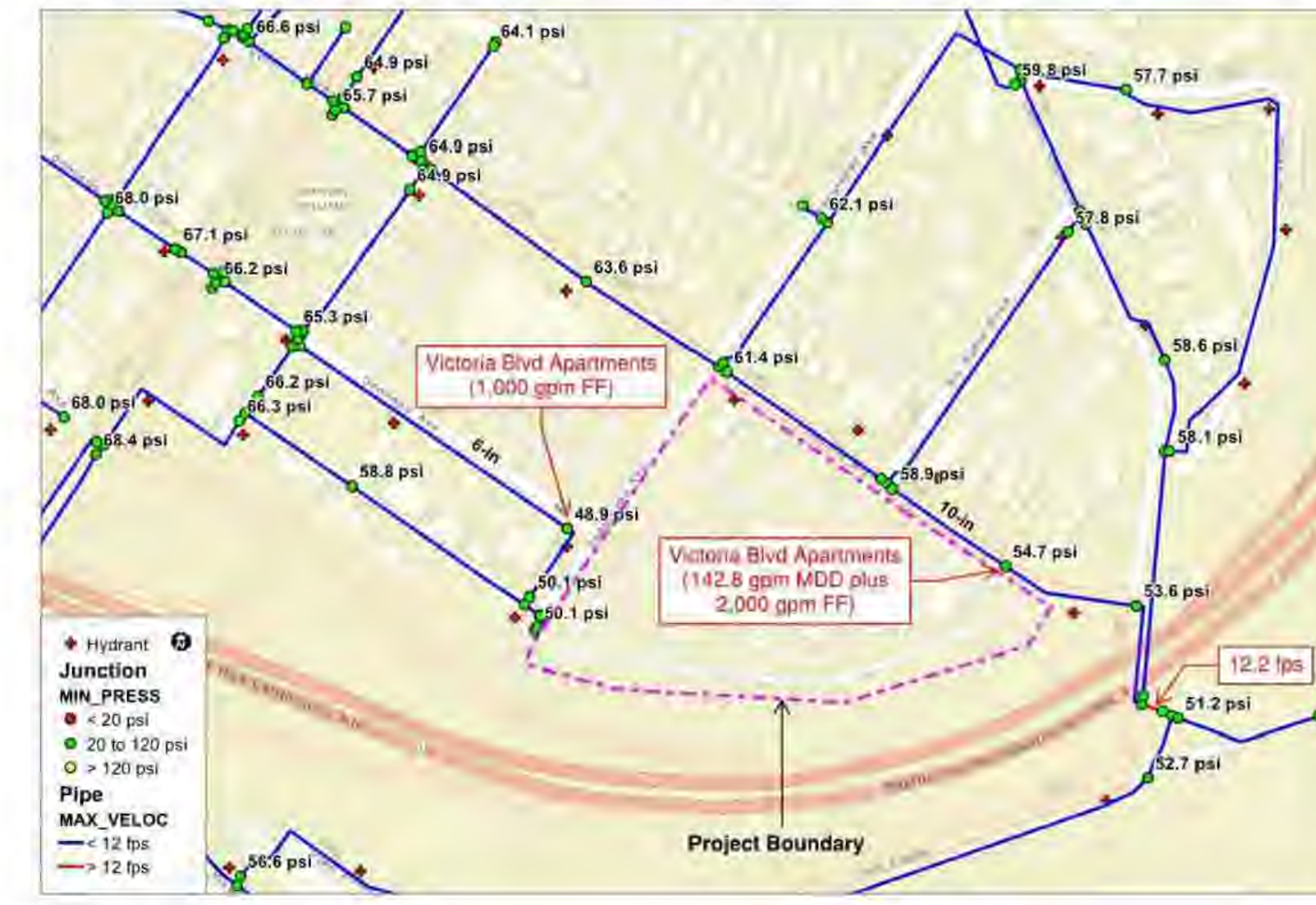
Figure 2-3: Run 2 - Existing (2020) MDD with Victoria Blvd Apartments MDD plus FF Results Analysis - Minimum Pressures and Maximum Velocities
