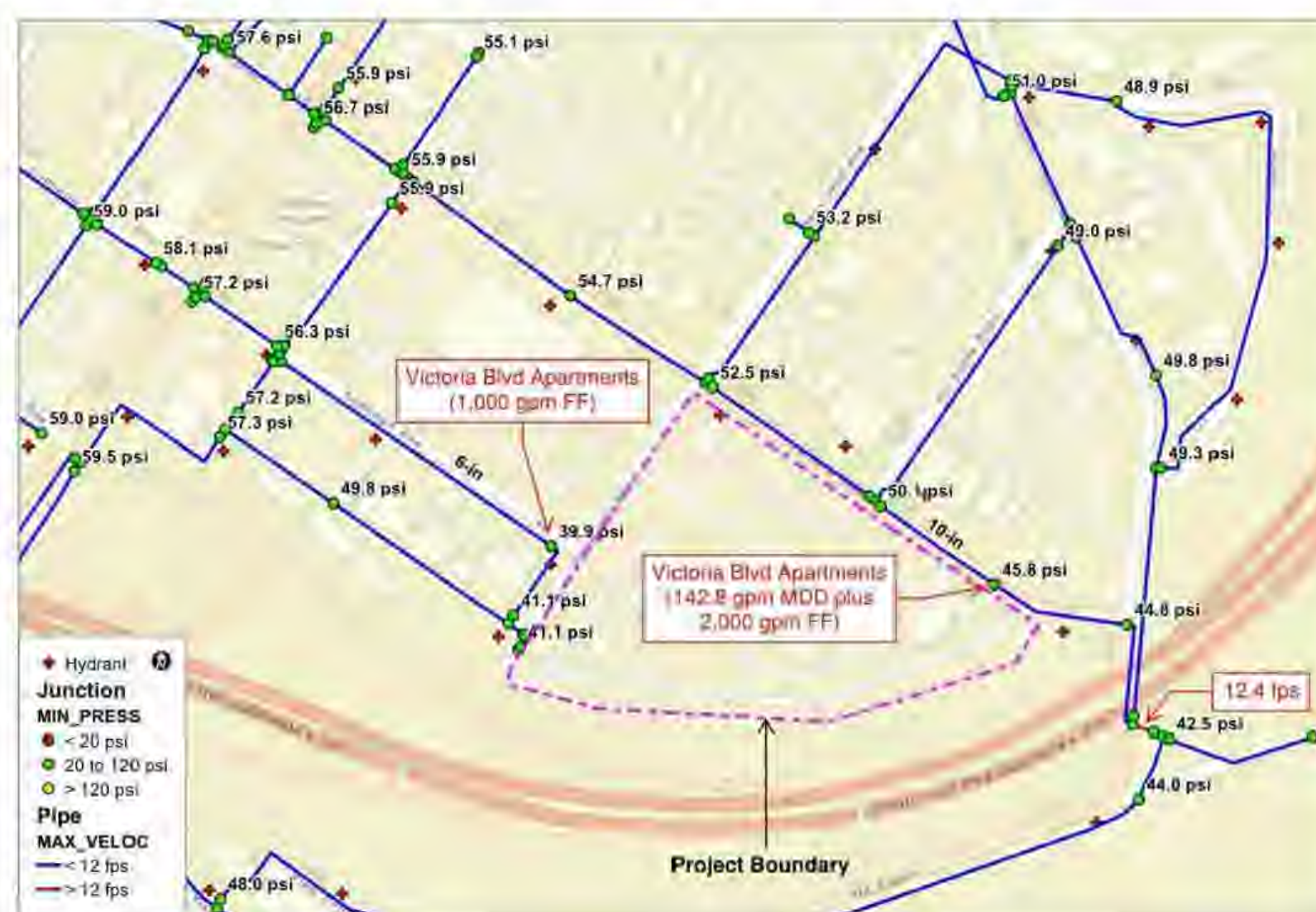
Figure 2-6: Run 2: Future (2040) MDD with Victoria Blvd Apartments MDD plus FF Results - Minimum Pressures and Maximum Velocities
