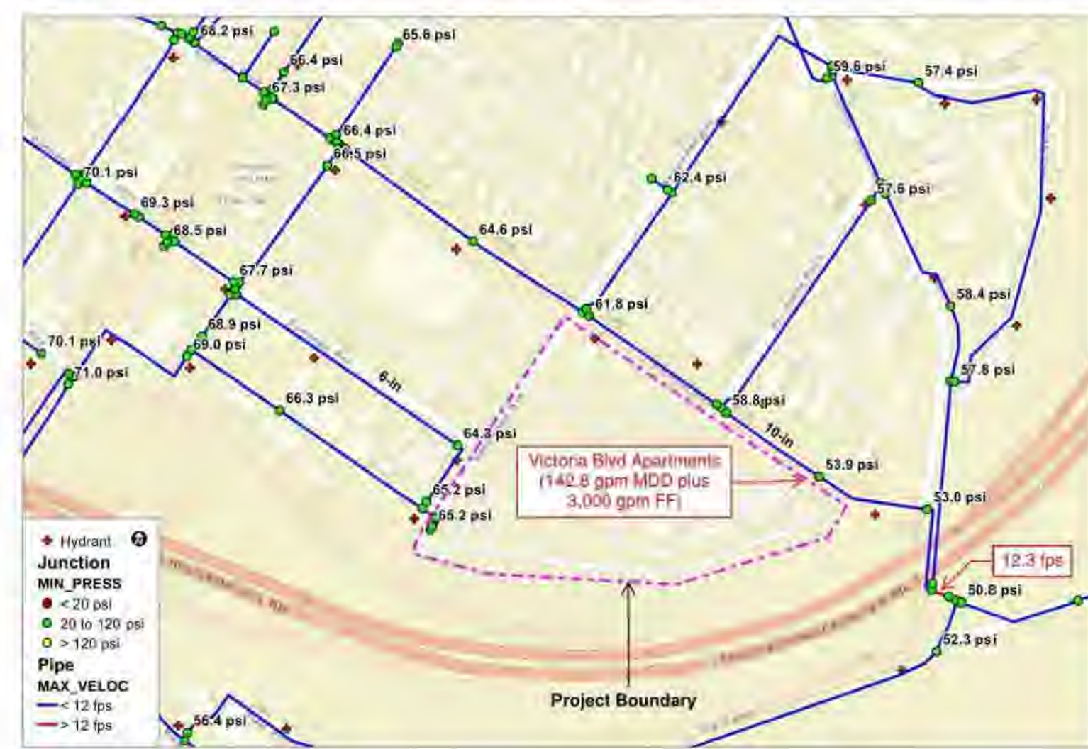
Figure 2-2: Run 1 - Existing (2020) MDD with Victoria Blvd Apartments MDD plus FF Results Analysis - Minimum Pressures and Maximum Velocities
