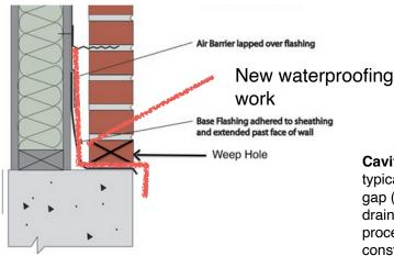
**Cavity Wall Construction**: Cavity walls are typically composed of two layers of masonry with a gap (cavity) in between. The gap is essential for drainage and ventilation. The waterproofing process should take into consideration the proper construction and maintenance of the cavity wall.
