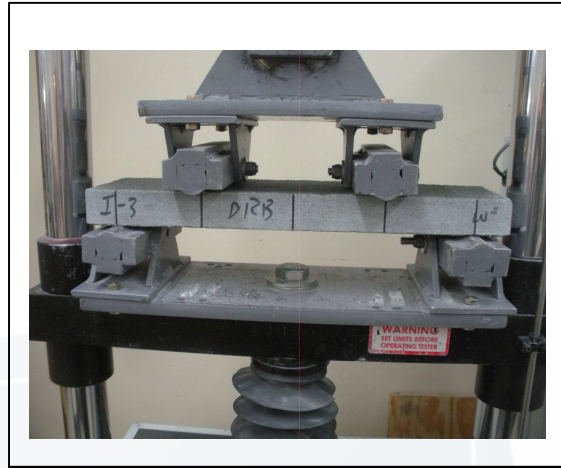
Photo No. 10 ASTM C880 – Specimen Loading Detail
