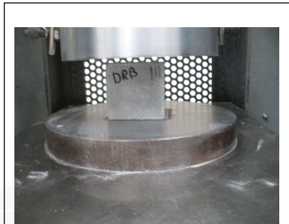
Photo No. 2 ASTM C170 – Test Setup
