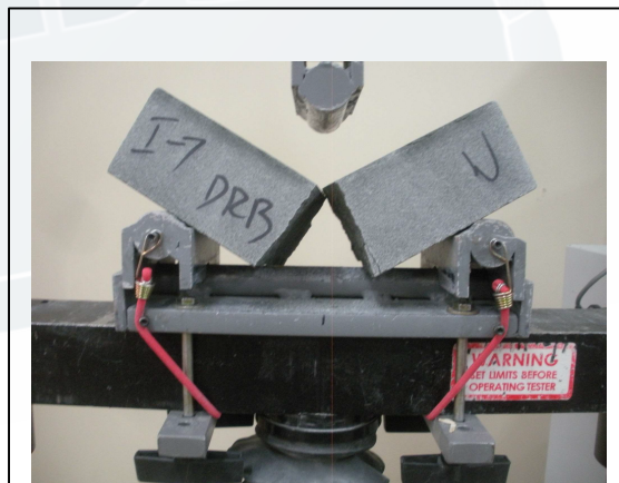
Photo No. 8 ASTM C99 – Specimen Failure Mode: Indeterminate Stone Rift (Wet Condition)
