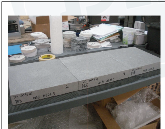
Photo No. 19 ANSI A326.3 – DCoF Test Set Up
