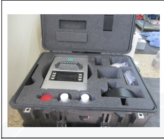
Photo No. 17 BOT 3000E Test Apparatus
