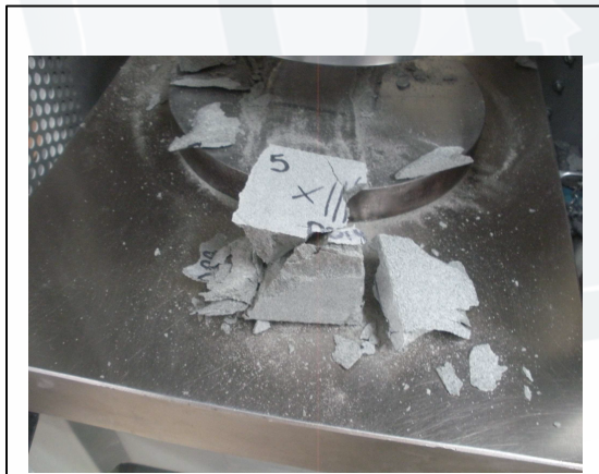
Photo No. 3 ASTM C170 – Specimen Failure Mode: Indeterminate Stone Rift, Side Loading (Dry Condition Depicted)
