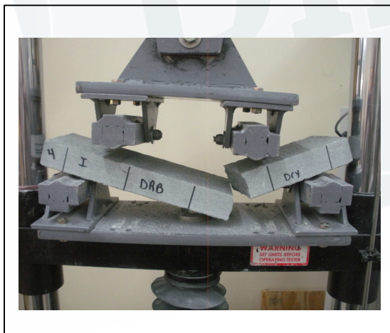
Photo No. 11 ASTM C880 – Specimen Failure Mode: Indeterminate Stone Rift (Dry Condition)
