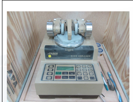
Photo No. 14 ASTM C1353 – Abrasion Test Setup
