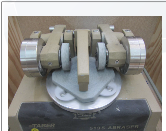
Photo No. 15 ASTM C1353 – Test in Progress
