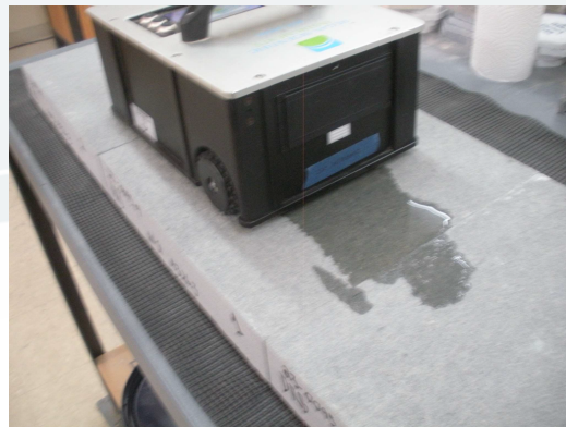
Photo No. 20 ANSI A326.3 – Test in Progress
