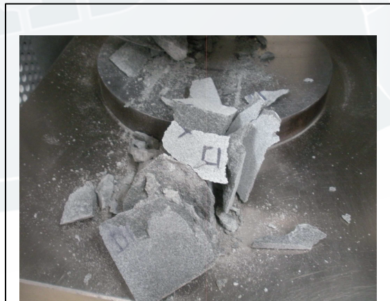
Photo No. 4 ASTM C170 – Specimen Failure Mode: Indeterminate Stone Rift, Face Loading (Wet Condition Depicted)
