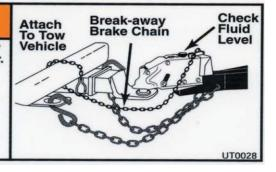
Trailer can roll if it comes loose. Electric safety brake applies when cable pulls pin out of switch box:
