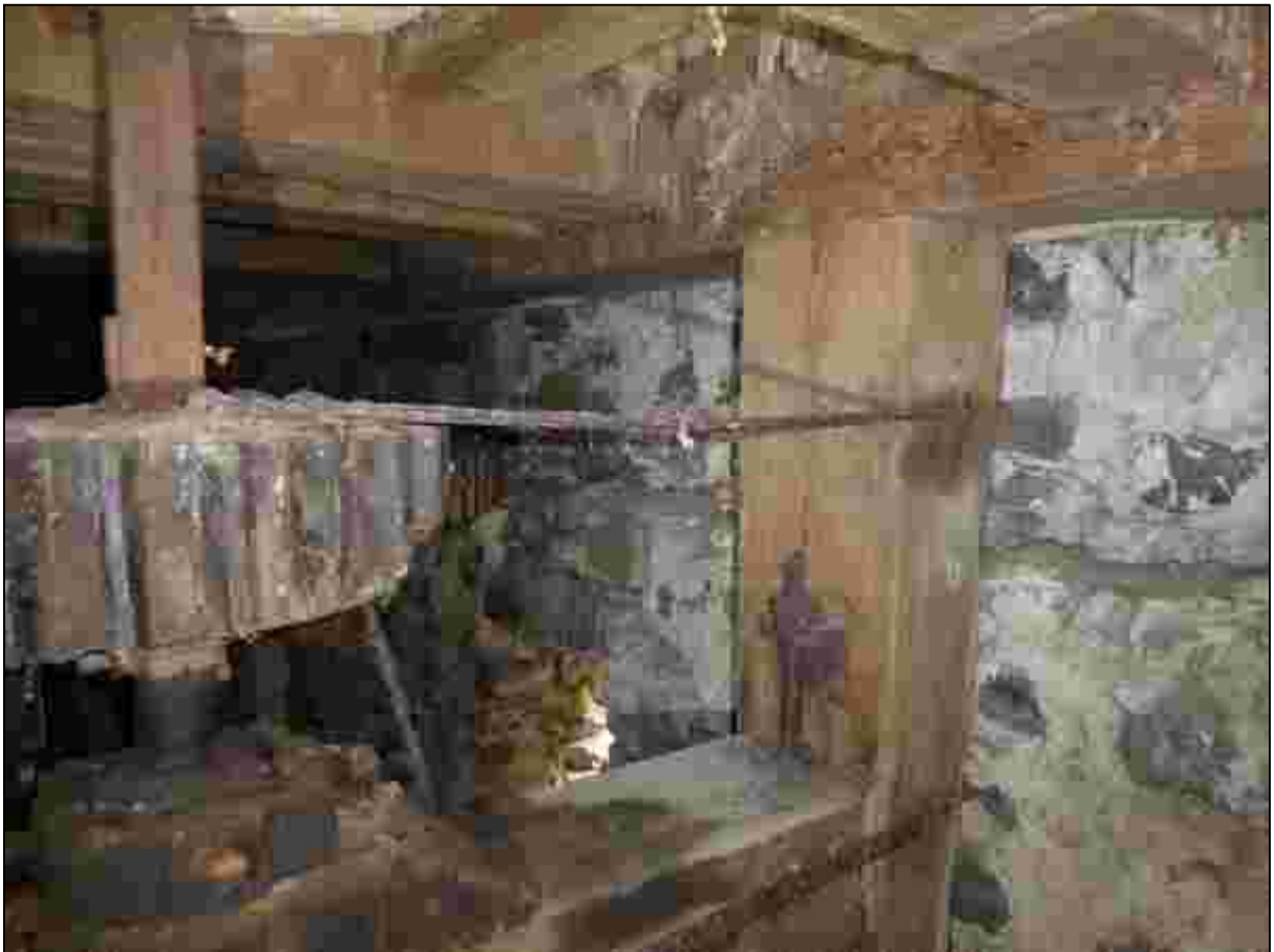
Plate 76: The latch securing one of the stone nuts and part of the tenting gear
