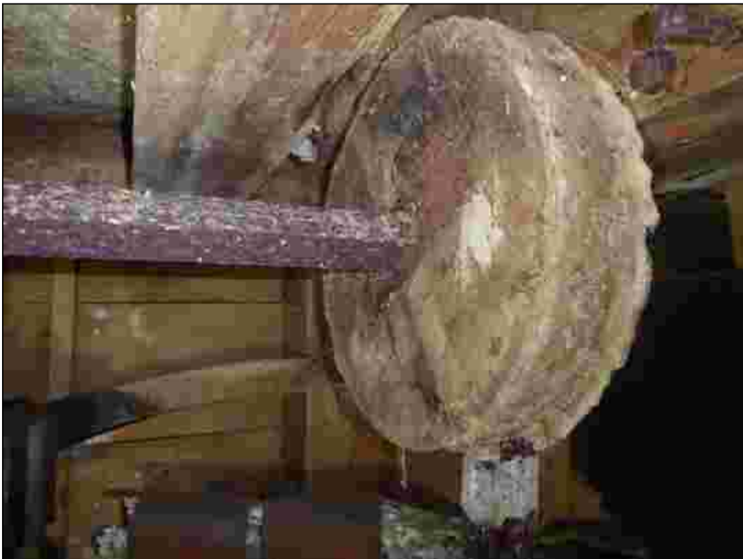
Plate 84: The pulley wheel on the lower lay shaft within the Hurst Frame
