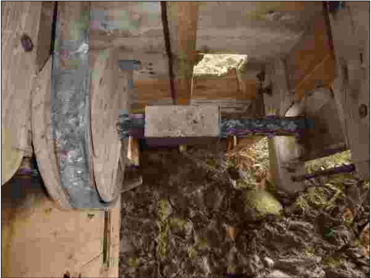
Plate 85: The second pulley wheel and third bearing block for the lower lay shaft
