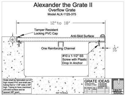
Grates exceeding 18" wide are fabricated with two reinforcing "C" channel, centered on the underside as shown below
