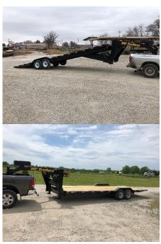
Powerful hydraulic power tilting trailer with low deck profile and gooseneck hitch std.
