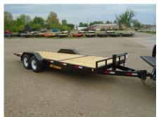
Beefy low-profile design with 6" channel steel frame and tongue system, plus 3" channel steel crossmembers on 16" centers. Adjustable height coupler std with your choice of coupler type or pintle ring hitch at no charge.
