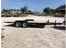
Every rugged item we ever designed into the HD flatbed but in an easy-to use manual hydraulic tilting trailer. Just pump up the jack to tilt it and when you get loaded, let it back down, tie down and go! Simple.
