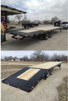
The original torque tube equipped hi deck trailer with its own hydraulic dovetail system. Torque tubes keep torsional twist to a minimum. Full 19 pound per foot wide flange 12" I beam frame, neck and tongue std. 3" channel crossmembers on 16inch centers always. Low profile 36" deck height std. Full 102" wide deck std. Adjustable height 2 5/16" gooseneck coupler with dual slide locks plus through neck locate pin for secure towing. 3/8" grade 70 safety chains with self-latching hooks.
