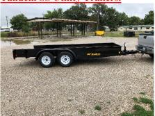
A proven design for 32 years. Full 7,000lb GVWR rating. 5,500lb in bed load capacity. 1,500lb max ramp capacity. Dexter brand easy lube axles. 3,500lb capacity each. Strong 6 bolt pattern hubs. 4-wheel electric brakes Brake breakaway system with on board battery and charger. New factory warranted ST205 75R-15 6 ply radial trailer tires. Strong Dexter steel mod wheels in white or black.
