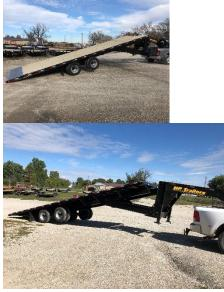
The original design power tilting deck over trailer! Just punch a button to tilt it up and another to tilt it down. Torque tubes keep torsional twist to a minimum. Full 19 pound per foot wide flange 12" I beam frame, neck and tongue
