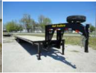
44' 20,000lb tandem dual unit shown with optional add on matching spare wheel and tire.
