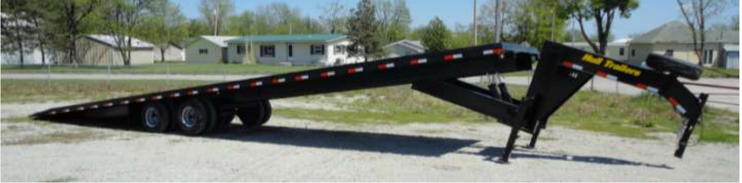
44' 20,000lb tandem dual unit shown with optional add on matching spare wheel and tire.
