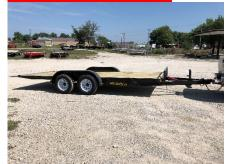
Every rugged item we ever designed into the HD flatbed but in an easy to use manual hydraulic tilting trailer. Just pump up the jack to tilt it and when you get loaded, let it back down, tie down and go! Simple.
