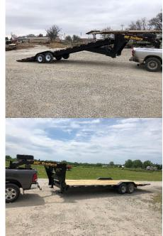
Powerful hydraulic power tilting trailer with low deck profile and gooseneck hitch std.
