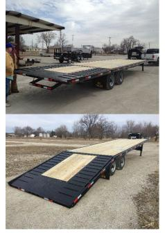
• The original torque tube equipped hi deck trailer with it's own hydraulic dovetail system.
