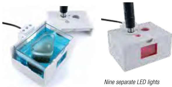
Dual chambers allow sample to set in temperature controlling water bath.
