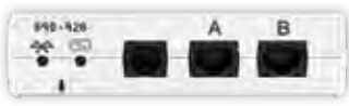
Wireless and rechargeable, the //control.Node has two ports for stepper motors, two ports for servo motors, and one port for digital sensors.
