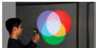
Use it as a projector in classroom demonstrations. Individually adjust the intensity of the super bright red, green, and blue LEDs.
