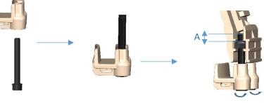
9. Keep screwing the M6 screws in small steps, each screw at a time until the main unit is with full, even and tight contact with the helmet and the unit doesn't move.
