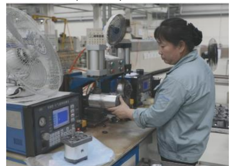
Air leakage inspection
