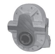
Flow Rate (gpm) = Displacement (in<sup>3</sup>/rev) X Speed (rpm) / 231 Volumetric efficiency ≥93%
