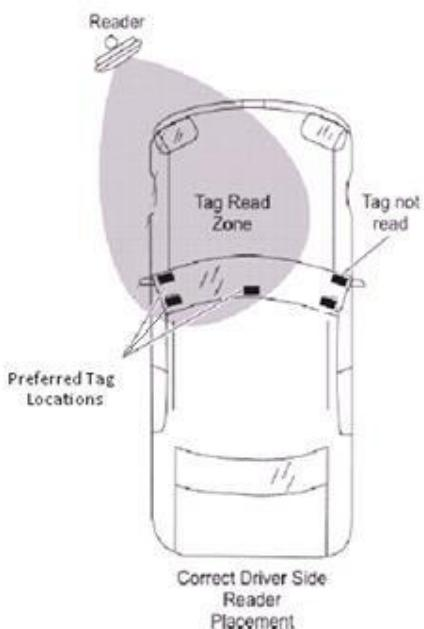
The diagrams below show suitable mounting locations of windshield tags. Choose a mounting location for the tag at least 2.5" from any materials containing metal. This includes the vehicle roofline, side pillars and rearview mirror mounting block.
