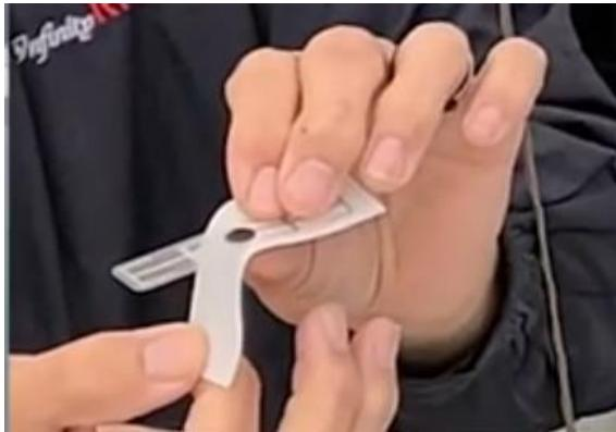
**Step 2** -Transfer the tag to the location on the vehicle that you have determined suitable for your application. It is best to apply the tag by the edges as shown in the picture below.
