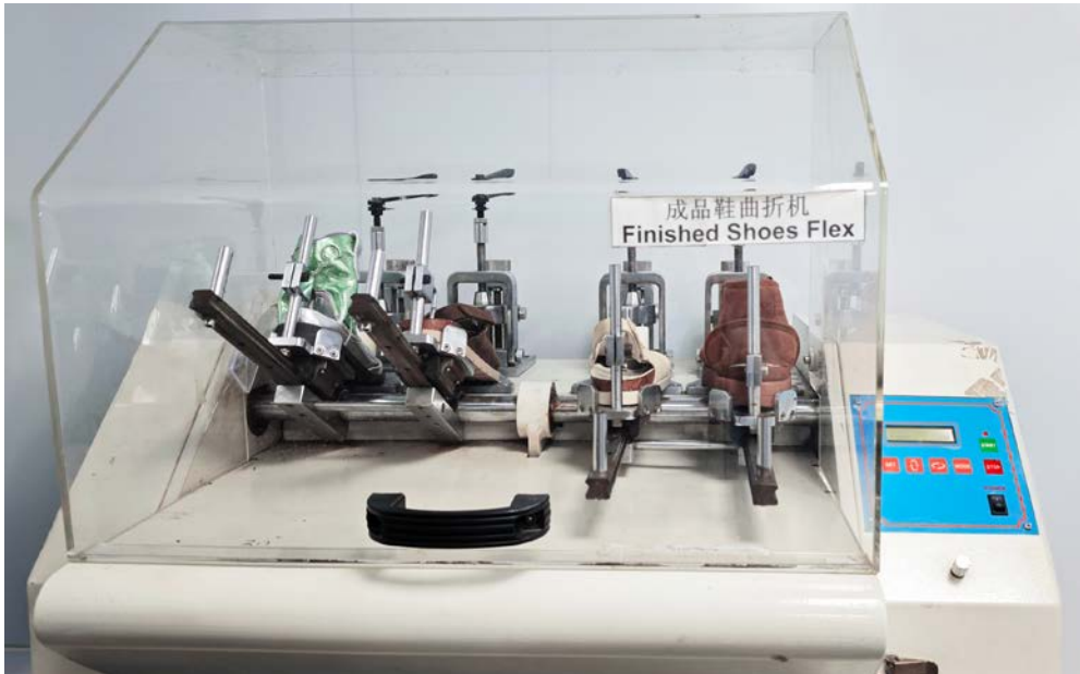
Finished Shoes Flexing Tester
