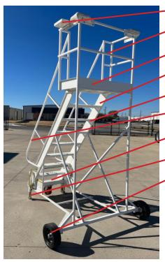
**90LNCTRLSTAND** affords a wide standing platform inside a safety cage to work on all high maintenance points on all types of rotorcraft with stability and safety. ANSI 14.7 OSHA 800 LB. \$6499.
