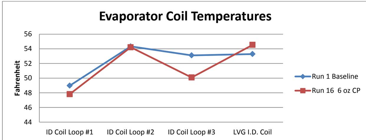
As part of the design of Cold-Plus® there are proprietary polymers that will not become a part of the boundary PTFE layer. These polymers circulate with the refrigerant and when they get to the evaporator they provide inert particles that aid in nucleation during the pool boiling phase. Simply put it is like water boiling at a lower temperature when you introduce a substance like salt. This change in pool boiling will lower the evaporator temperature and allow for more efficient operation.
