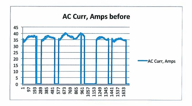
This is the data for before injection. You will note that the system starts and runs almost continuously until it reaches the set point where it cycles off until the ambient rise causes it to turn on and repeat the cycle. This is characterized in the graph. Run amperages are from 34 to 41 amps.
