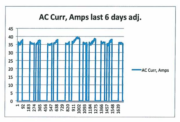
You can clearly see a different pattern here after the Cold-Plus™ injection, the unit cycles when the thermostat setting has been met and spends considerably more time with the compressor not running.
