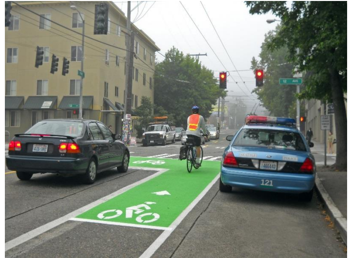
Bike boxes and green pavement (combined in this example) are two tools for improving intersections for bicyclists. Bike boxes improve the ability for bicyclists to make left turns at intersections.
