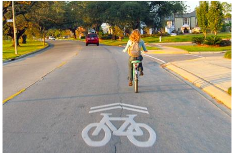
Shared lane markings show preferred lane positioning to people bicycling while also reminding drivers to expect people on bikes.
