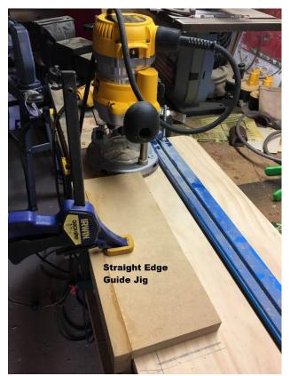
Using a long metal straight edge, I clamped it to the piece to use a stop for the router.
