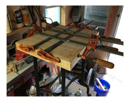
After the glue dried I unclamped the assembly and smoothed up the outer edges.
