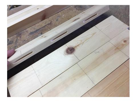
With the biscuit holes cut I lined up all the boards on top of some clamps. Then I used scrap pieces of wood where the clamps will come into contact, so they wouldn't crush, or disfigure, the "good" wood.
