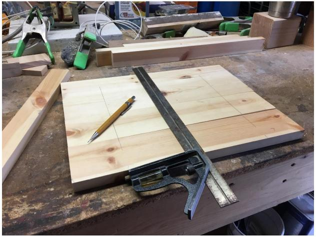
I cut the boards to the desired length and ripped them to achieve the dimensions that I needed. Next, I drew lines using a straight edge to mark where to plow the biscuit joiner.
