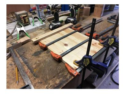
I clamped everything together and turned the assembly over and clamped it to my work bench to prevent warping.
