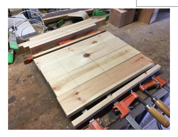
Next I applied a liberal amount of wood glue along the entire edge surfaces, as well as in the biscuit cutouts. Inserted the biscuits and assembled the pieces.
