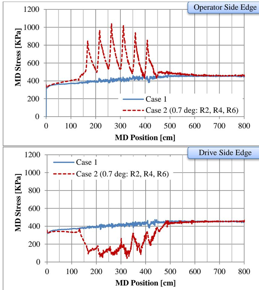
**Figure 6: Comparison of MD stresses in the web along its length at different CD locations between Case (1) and Case (2)**
