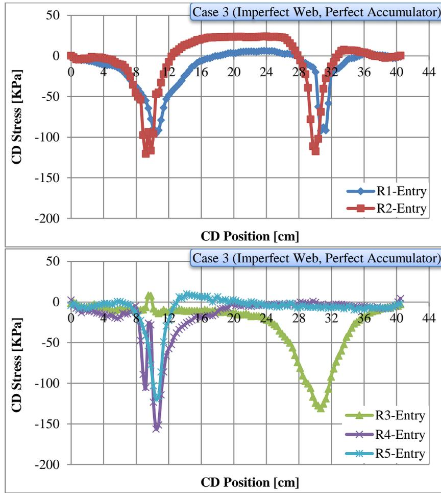
Figure 12: CD stresses due to web imperfections at the entry of rollers R1-R5.
