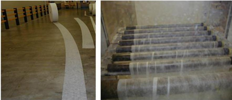
**Figure 1: Cambered web and wrinkles in an accumulator**
