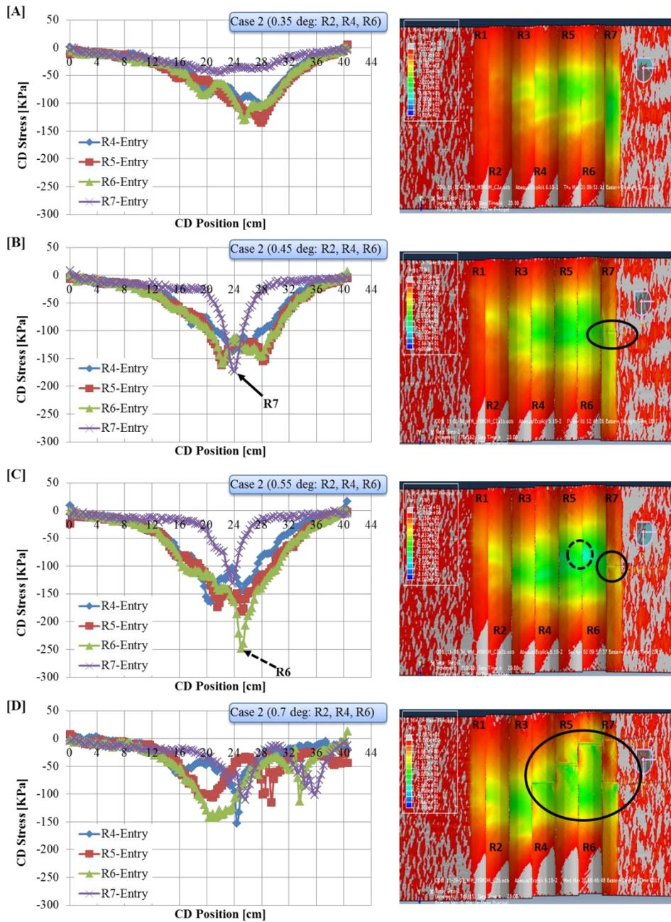
Figure 7: CD stresses in the web at the entry of rollers R4-R7 and contours of CD stresses in the web for rollers R1-R7.
