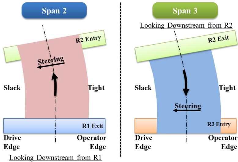
**Figure 9: Schematic of web behavior in spans 2 and 3.**
