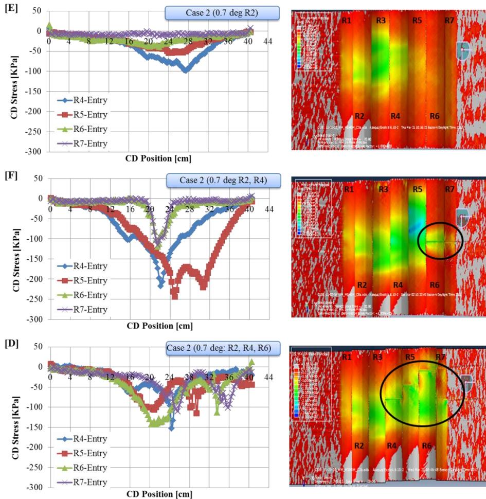
**Figure 8: Comparison of CD stresses for cases wherein one, two or all three top carriage rollers are misaligned. [Case 2(d) is included for comparison purposes and contains the same data as presented in Figure 7[D]]**
