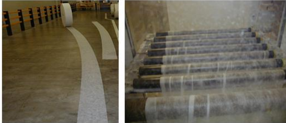
Figure 2 – Cambered Web & Wrinkles in the Accumulator
