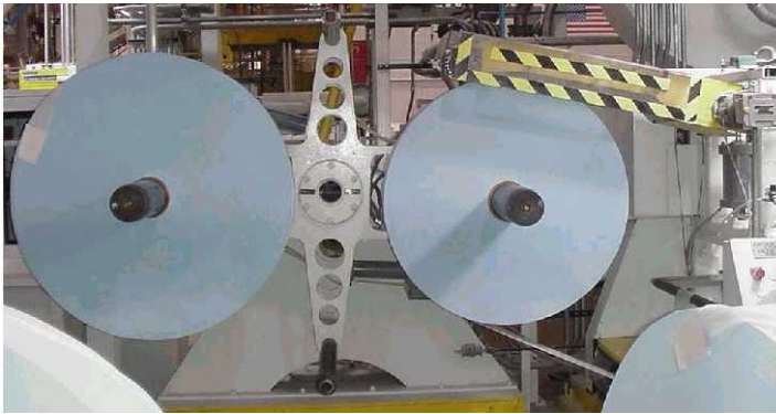
Turret with Surface Drive Belts
