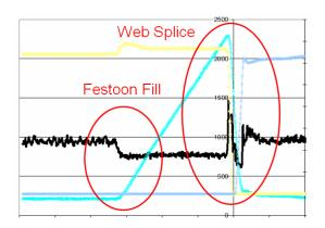
There are two important time periods of interest. The first is when the unwind begins to fill the festoon. The festoon fill phase is the first departure from steady state conditions. It is common to see troughs in open spans and wrinkles across rollers to appear. The second time period of interest is the splice itself. A lot of things take place in a very short period of time. It is important to sort thru the details to better understand what you are looking at.
