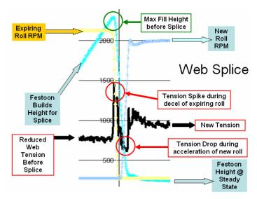
The web tension is black. The festoon height is shown in light blue. Note that before the festoon begins to raise that the tension was in steady state. At the same time the festoon begins to raise the web tension drops a significant amount to a new steady state condition. Recall that the expiring roll is accelerated to a new (higher) speed to fill the festoon. The web is driving the idlers. The web has to give up tension to accelerate the idlers.
