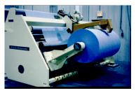
A more sophisticated start/stop unwind will drive the roll to provide for tension control. Often this is done with a surface drive belt like the one shown to the left. Note that this unwind also provides for chucking and lifting the roll from the floor. Both of these unwinds will require the machine to come to a complete stop to load a new roll.
