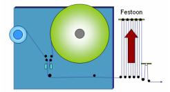
As the expiring roll triggers the splice sequence the spindle drive will be accelerated to a higher speed.
