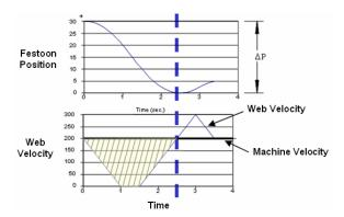
The timing of the splice and the storage requirements for the festoon are often mapped using graphs of festoon position and web velocity. This allows one to determine requirements for festoon capacity based on acceleration and deceleration rates.
