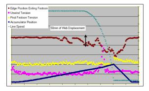
Wide processes are negatively impacted by width loss. Narrow processes are negatively impacted by web weave. All processes are negatively impacted by wrinkles. All three of these can be detected with a combination of web width sensors and cameras. An analog signal from your sensors can be imported into your trend charts as shown to the left.
