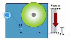
The next step is to decelerate the expiring roll to a complete stop. The splice will then take place. As the splice bars open up the new roll is accelerated to back to nominal web speed.
