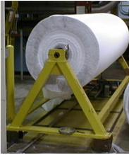
A simple unwind stand is often used to provide a web to a process but will be limited in speed. The addition of a drag belt is often used to slow down the roll when the machine stops.
