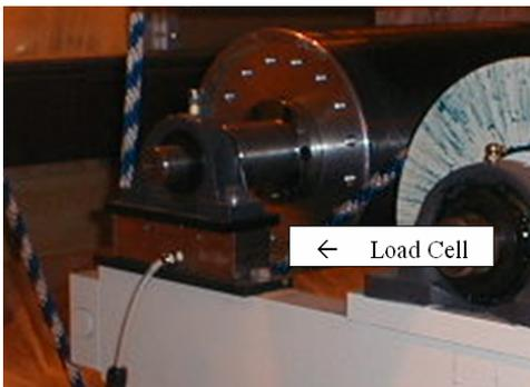
The best way to understand your web process is to directly measure the web tension. Cantilevered load cells are often used for narrow webs. Wide web processes normally mount an idler mounted on top of load cells. It is important for the load cell roller to very well balanced (G1.0 or better) and mounted properly to avoid machinery vibration.
