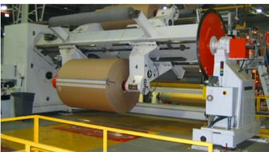
As the roll grows in size & weight drives are added to the spindles to bring the roll to web speed as shown on the unwind to the left. Spindle drives are also ideal for rolls that are slippery or would be damaged by direct contact with the surface belt.
