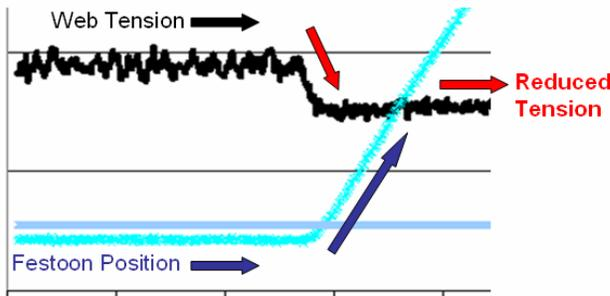
The web tension is black. The festoon height is shown in light blue. Note that before the festoon begins to raise that the tension was in steady state. At the same time the festoon begins to raise the web tension drops a significant amount to a new steady state condition. Recall that the expiring roll is accelerated to a new (higher) speed to fill the festoon. The web is driving the idlers. The web has to give up tension to accelerate the idlers.
