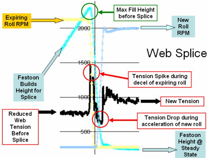
This graph details the splice event. Recall that the splice is accomplished by decelerating the expiring roll to a complete stop. It is during this time that the tension spikes. The spindle drive is stopping the roll. The web from the roll is trying to stop the idlers. At the same time the moving carriage is being pulled down by the web. Once the roll has been stopped the splice bars close to make the splice. The moving carriage continues to be pulled down as the downstream
