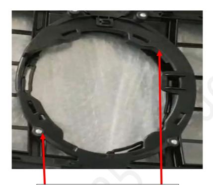
Arrowed is the circular radar unit bracket (you can see it is fixed with 3 fasteners. It important your grille has this, or else it is basically scrap plastic. Inspect the video below.
