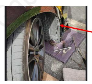
The parking sensor loom connector is just here (on inside of bumper)
