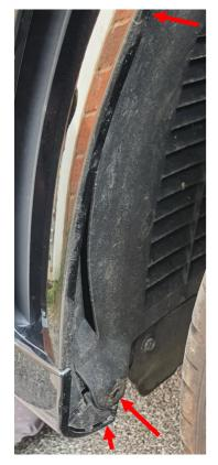
Remove the plastic push rivets from the outer edge of the arch liner, and 1 under the outer edge of the bumper, arrowed red. Use the body trim tools on pop rivets. Pull the centre of the rivet out then pull the main rivet.
