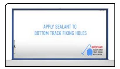
When you are completely satisfied that the track is level, fix the bottom track adjacent to the packers, ensuring that silicone is applied into the drill holes.
