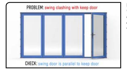
If the Swing Door is clashing with the keep door, check that the swing door is parallel to the keep door, if not check the level of both doors both vertically and horizontally.
