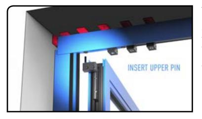
Then insert the previously removed upper pin assembly into the pivot hole on the top track and offer the panel to the pin assembly and reattach the fixings using the 3/16" allen key previously mentioned. Don't use power tools to attach the assembly.
