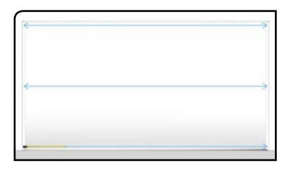
When measuring the opening sizes, it is important to take three horizontal measurements: bottom, middle and top.
