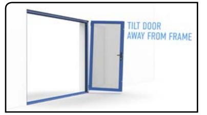
Utilizing two people, position the swing door at right angles to the frame close to the bottom pivot hole of the track. The door handle side should be farthest from the frame. Tilt the top of the panel away from the frame, then carefully lift the panel to allow location of the bottom pin on the panel into the bottom pivot hole of the track.
