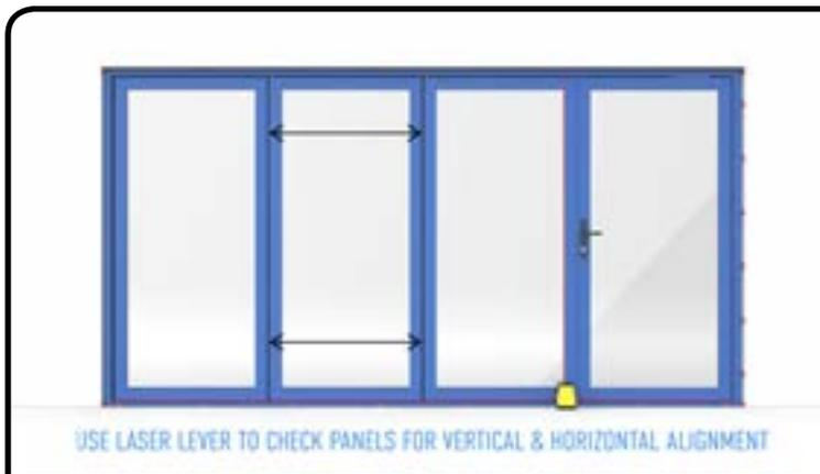
If any panel is not level, check that the width of the panels are consistent.
