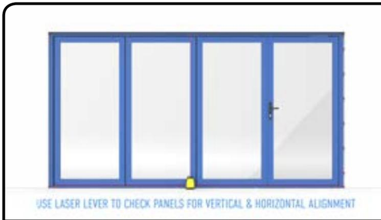
At this point check that all panels are square in the track. Check along the bottom of each panel and up one side using a laser level.
