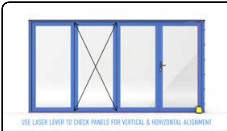
Check that the panel is square by measuring corner to corner on each side.
