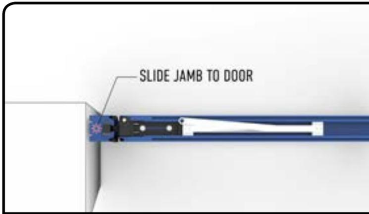
When the swing door is plumb, then the jamb next to the swing door can be set in position and fixed.
