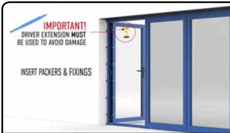
Ensure packers are positioned next to the fixing points and that they are not causing a twist in the jamb position. Take care when fixing the jamb not to damage the side of the swing door. We recommend an extension bar to keep the drill chuck clear of the swing door panel.
