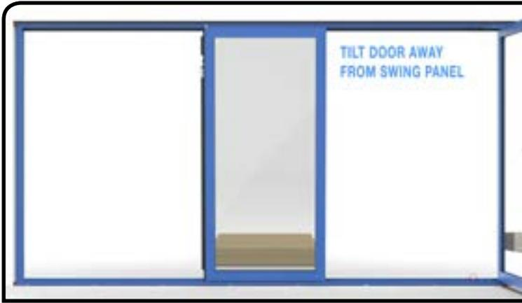
With the panel still not engaged in the top track, tilt the door away from the swing door
