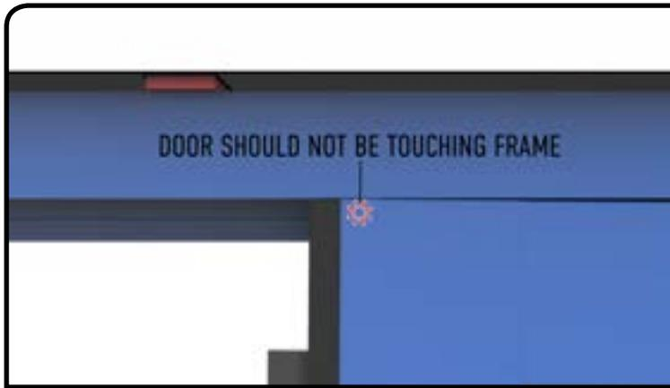
At this point there should be a 1/8" gap between the top of the door and the top track. By depressing the finger bolt you should feel the door open without resistance.
