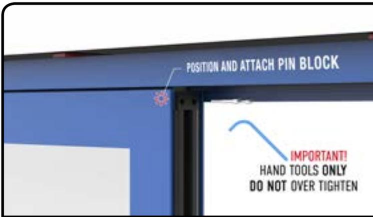
Fix using two 3/16" allen bolts. Hand tighten only. You may need to carefully lever the section attached to the magnet down using a non metallic lever like a glazing paddle to align with the panel block.
