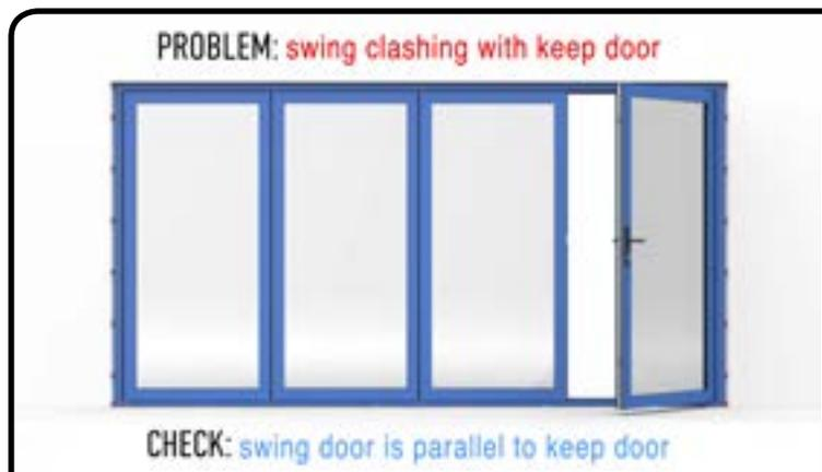
If the Swing Door is clashing with the keep door, check that the swing door is parallel to the keep door, if not check the level of both doors both vertically and horizontally.
