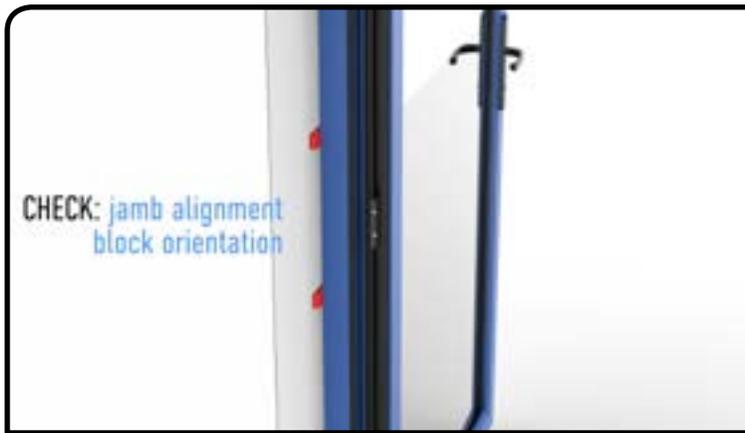
Also check that the orientation of the jamb alignment block is correct.
