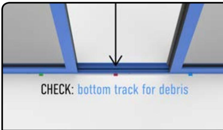
Check if any fixings are inhibiting the movement of the door.
