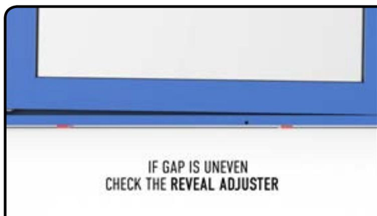
If that gap is inconsistent, check that all four reveal adjusters are fully retracted.
