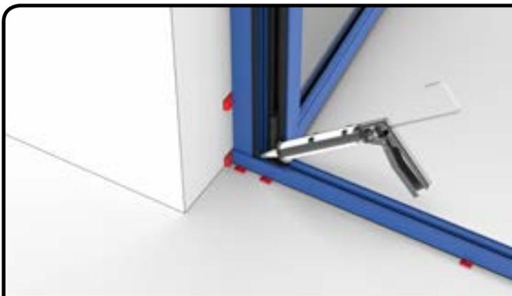
And finally, silicone seal beneath both door jams.
