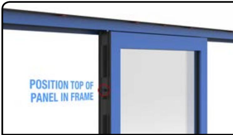
To position the panel into the top track, pull down the finger bolt and push the panel into the top track and release the finger bolt. Ensure that the latch is located in the top track before releasing.
