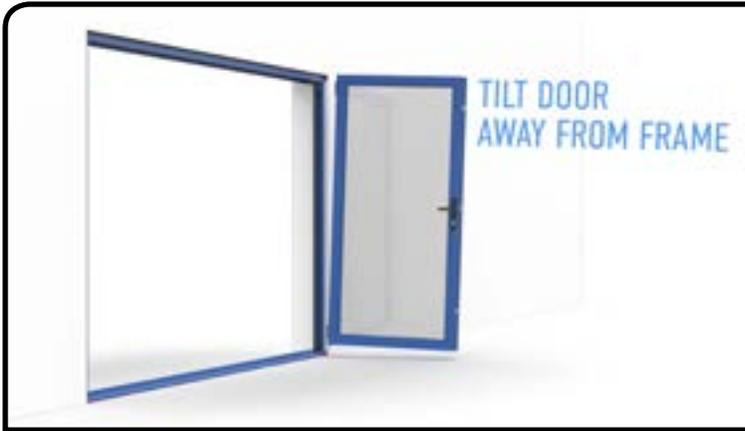
Utilizing two people, position the swing door at right angles to the frame close to the bottom pivot hole of the track. The door handle side should be farthest from the frame. Tilt the top of the panel away from the frame, then carefully lift the panel to allow location of the bottom pin on the panel into the bottom pivot hole of the track.
