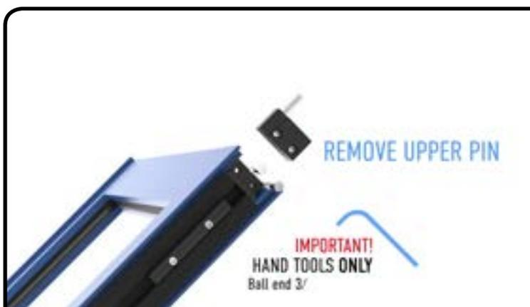
On the hinge side of the door, the upper pin assembly should be removed by undoing the two bolts using a ball end 3/16" allen key. Please note, no power tools should be used in either removing or fitting these assemblies at the top of each panel.
