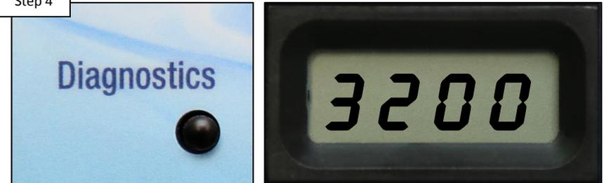
After 30 seconds the unit should settle back to the default reading. The reading should now reflect a number in thousands.
