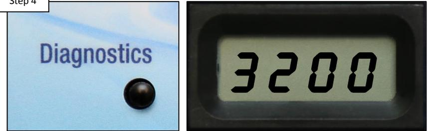
It takes about 30 seconds for the unit to settle back on the default reading. It should now reflect the average salt level.
