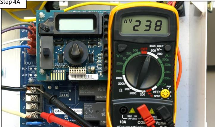
Test incoming power for 120/240VAC (+/- 15%). IF no/low voltage, then the problem resides in the power source and NOT the AquaRite control center. IF power is correct, go to step 4B.
