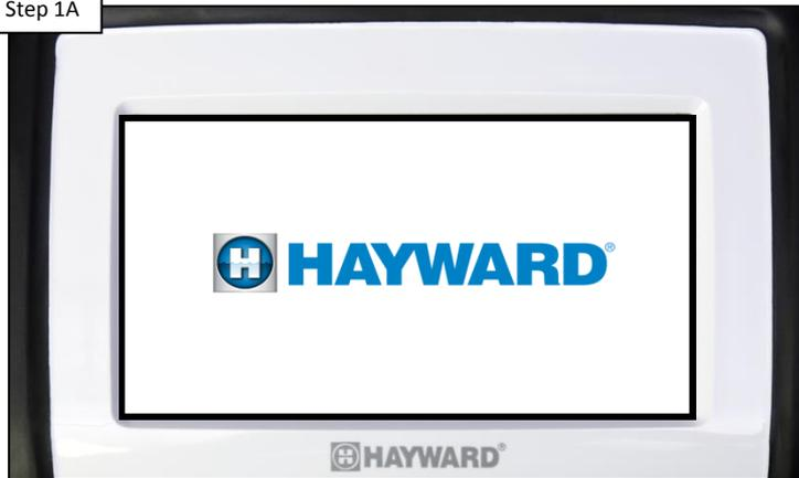
Tap on the controller screen in an attempt to wake the display from a system shutdown. Make sure glare is not the culprit. IF tapping does not change the display state, go to step 1B.
