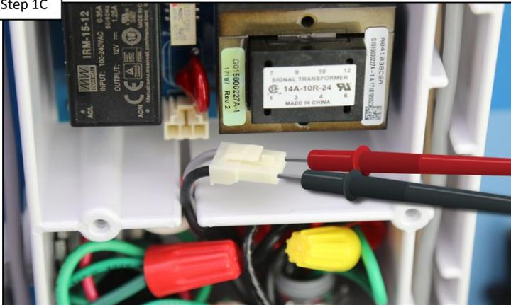
**Unplug input power connector. Verify 120 or 240vAC. IF 120/240vAC is present, replace the hub PCB (HLXHIOPCB). IF not, go to step 1D.**
