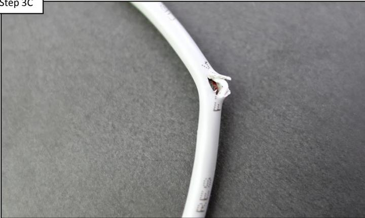
Inspect the Controller Wiring. IF the wiring is damaged replace the cable ([HLX485100](#)). IF the Controller wiring is not damaged, proceed to step 3D.
