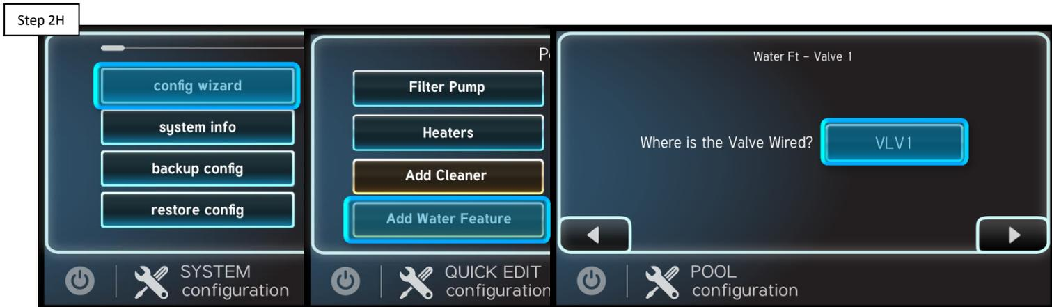
Using quick edit, reprogram the valve. IF the valve still will not rotate while being activating through the controller, then please contact support (908) 355-7995 for additional support.
