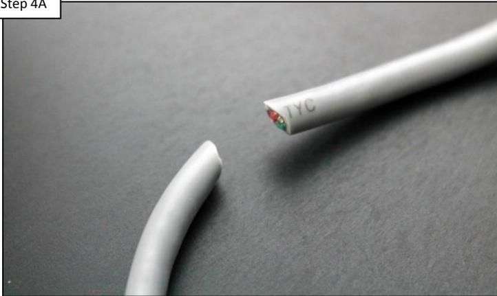
Inspect the Smart Relay cable for damage. IF no breaks exist and/or connections are correct, go to step 4B. IF comm cable is damaged, replace cable and retest ([HLX485100](#)).
