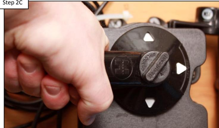
**Verify the actuator shaft is engaged (as shown above). IF the valve moves freely, when rotating the handle, pull up on the handle to engage, IF engaged, proceed to step 2D.**
