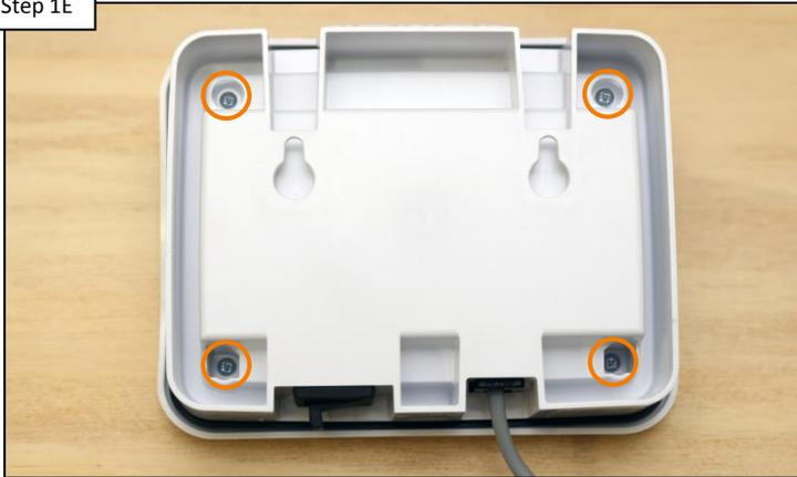
On the back of the controller, remove the 4 screws that secure the controller display to the housing. This provides access to the controller PCB. Once complete, go to step 1F.
