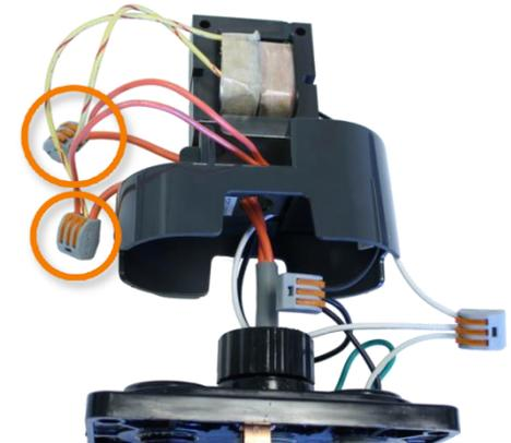
Open lighting transformer and test for 14vAC on the output side. IF voltage is correct on the output side of the transformer, replace defective lights. IF no/low voltage, go to step 7E.
