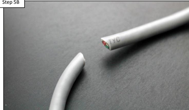
Inspect the pump's comm cable for damage. IF no breaks exist and/or connections are correct, go to step 5C. IF comm cable is damaged, replace the cable and retest.
