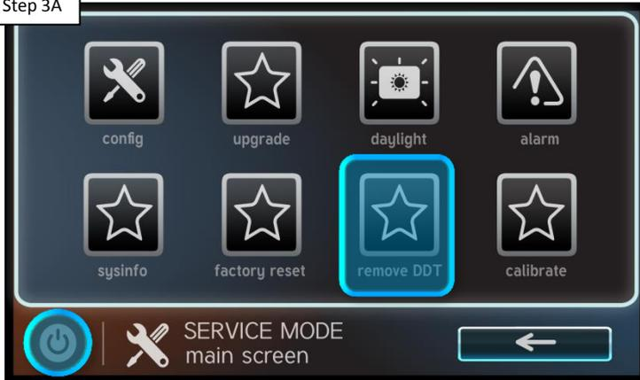
Follow steps to remove DDT (pg. 17). IF after programming is reestablished, the problem still persists go to step 3B. IF problem is corrected Backup configuration (pg. 14).
