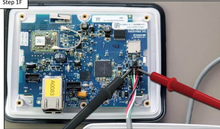
Test cable that plugs into controller PCB for 12vDC between terminals 1 & 3 (left to right). IF power is present, replace controller ([HLHCONTROL](#)). IF no/low voltage replace controller cable ([HLX485100](#)).
