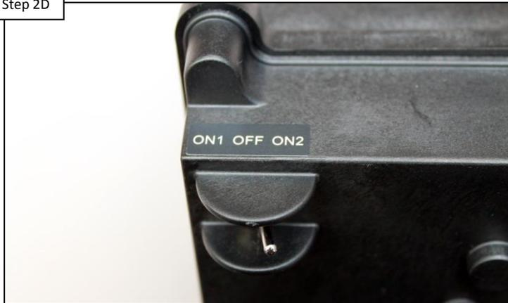
Locate toggle switch (bottom of actuator). Verify switch is either in ON1 or ON2 positions. Toggle the switch between ON1/ON2, IF actuator does not move, go to step 2E, otherwise skip to step 2G.
