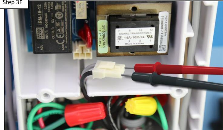
Unplug input power connector. Verify 120/240vAC. IF 120/240vAC is present, replace the hub PCB ([HLXHIOPCB](#)). IF no/low, resolve at the breaker/timeclock.
