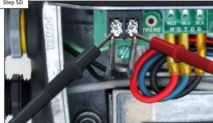
If pump is not powered, it will not be able to communicate with VS Omni. Verify pump has 187-253vAC. IF no/low voltage, resolve at pump breaker. IF correct please contact support (908) 355-7995\*.
