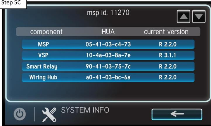
Navigate to Config>System Info and verify the Pump HUA is showing up in the list. IF HUA does not appear, go to 5D. IF it does, reprogram VS Omni, contact support if the problem still persists: (908) 355-7995.
