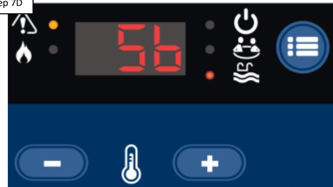
“Stuck Button” indicates display board is acting as if the button is being pressed and held. Replace display/bezel/key pad (pg. 25).
