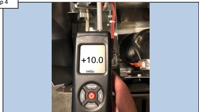
Leave the heater in "Stand By", your static pressure should be no less than +4.0 and no greater than +14.0" WC.
