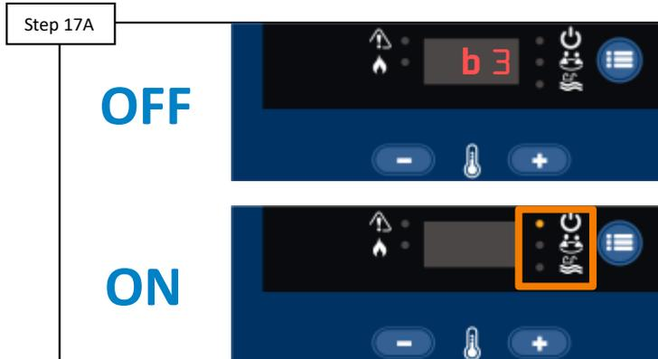
Power cycle heater, in an attempt to clear the “b3” code. IF power cycling clears to the “b3” message and the heater fires, drop the temperature to suspend heating. IF “b3” reappears, go to step 17B.
