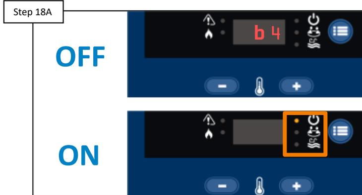
Power cycle heater, in an attempt to clear the “b4” code. IF power cycling clears to the “b4” message and the heater fires, drop the temperature to suspend heating. IF “b4” reappears, go to step 18B.
