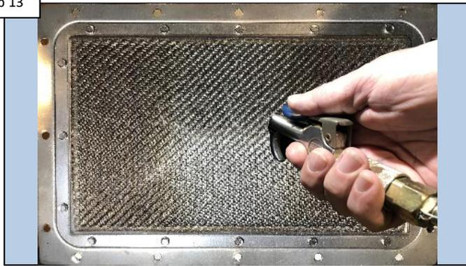
Using compressed air blow the burner out from the front to the rear. Make sure that you blow around all four corners.
