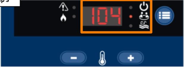
The 'SPA' indicator will flash & the display should show the Max Temp set point.
