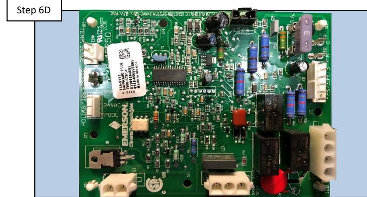
IF after replacing display/bezel/keypad, “CE” error persists, replace ICB (pg. 25). IF replacing ICB fails to solve problem, contact support (908) 355-7995.
