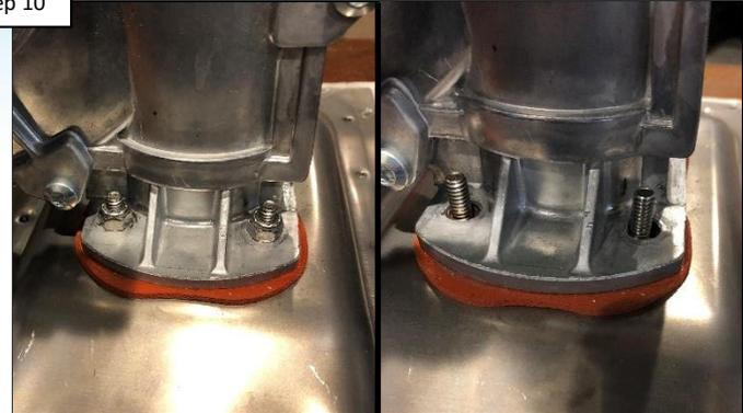
Remove the 4 each 7/16" nuts that hold the blower assembly to the burner.
