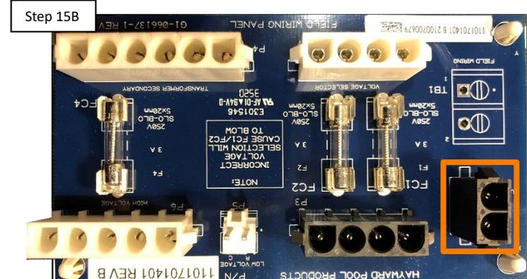
Unplug the wire harness from the P1 terminal and test voltage on the harness (115VAC or 230VAC). IF incoming voltage is out of range (+/-10%), correct incoming voltage. Otherwise, replace the ICB (pg. 25).
