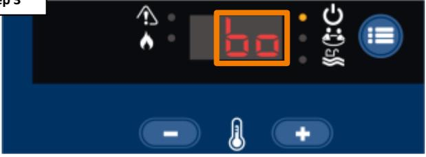
'bo' will appear on the display when the heater has successfully entered bypass operation.
