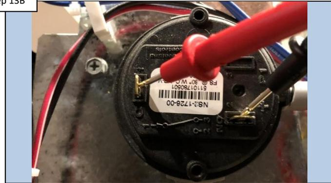
**Isolate the diff. pressure switch. Measure continuity between switch terminals. IF continuity exist, replace the blower vacuum switch (pg. 25).**
