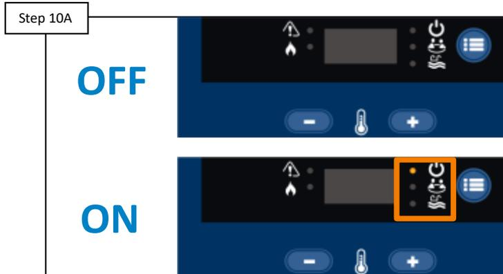
Power cycle the heater, in an attempt to clear the “HF” code. IF power cycling clears to the “HF” code and the heater fires, drop the temperature to suspend heating, IF “HF” reappears, go to step 10B.
