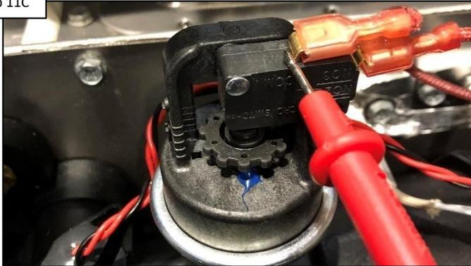
Next take the other lead on your multi-meter and test for 24V AC on one of the terminals on the water pressure switch, then Go To Step 11D.
