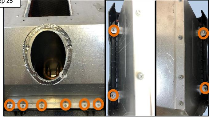
Remove the 6 screws at bottom of combustion chamber. Remove 2, 7/16" nuts on each side of chamber (right pics). Remove combustion Chamber.
