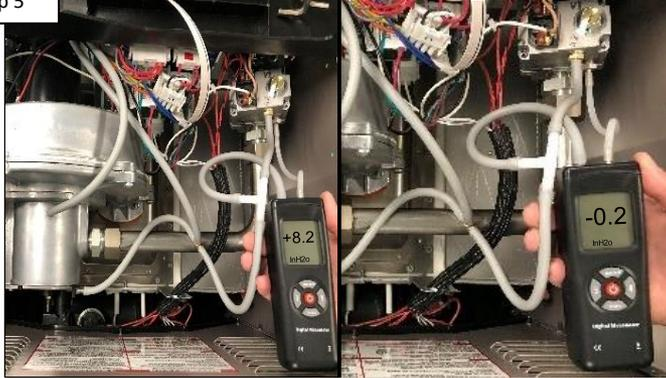
Once the manometer is connected, turn gas back on & test inlet & manifold gas pressures. Go to Step 6.
