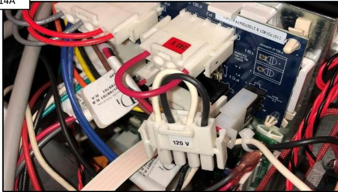
Verify selector plug matches incoming line power. IF it does not, power OFF & correct. IF OK, go to Step 14B.
