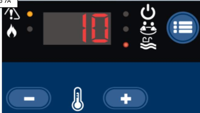
“IO” error indicates ignitor open. IF this error appears, go to step 7B. IF “IO” does not appear, go to step 7D.
