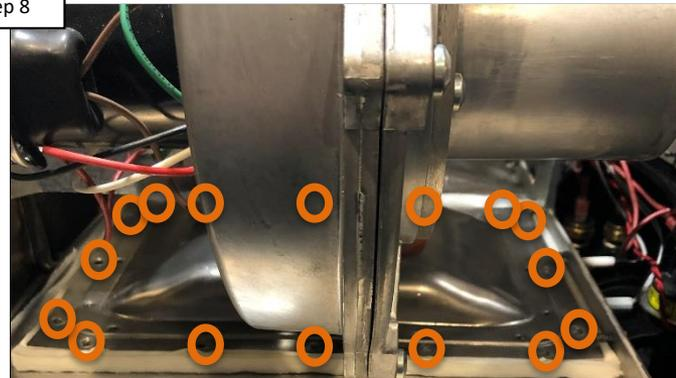
Remove the 16 screws from the burner to release the entire blower and burner assembly.
