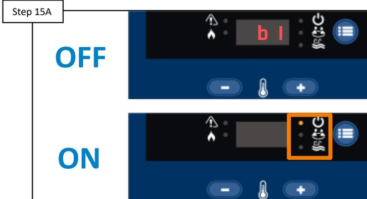
Power cycle the heater, in an attempt to clear the “b1” code. IF power cycling clears to the “b1” code and heater fires, drop temperature to suspend heating. IF “b1” reappears, go to step 15B.
