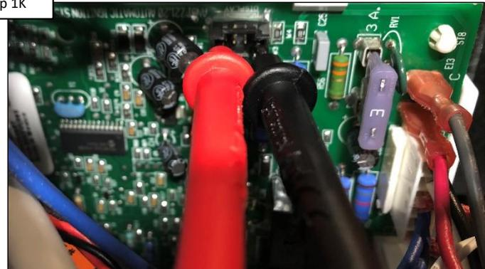
On the ICB, verify 22-28VAC between AC & COM terminals (pins 1 & 4). IF voltage is present, replace display/bezel/keypad. IF no voltage, replace ICB (pg. 25).
