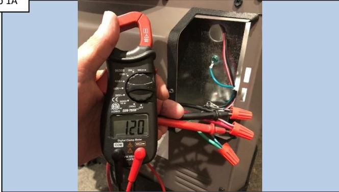
IF voltage is present, go to step 1B. IF voltage is incorrect, correct source power.
