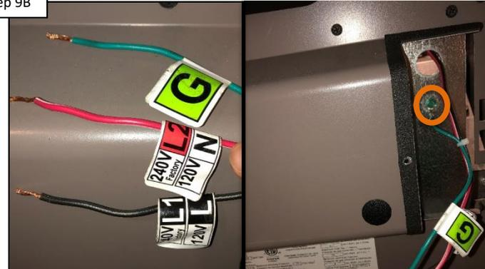
Verify both neutral and ground connections (both internal and external) are clean and secured. IF ground and neutral connections check-out, then replace the ICB ([pg. 25](#)).
