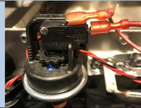
With power off, inspect the water pressure switch wiring for damage. IF damaged, replace the wire harness (pg. 25). IF OK, go to step 3C.
