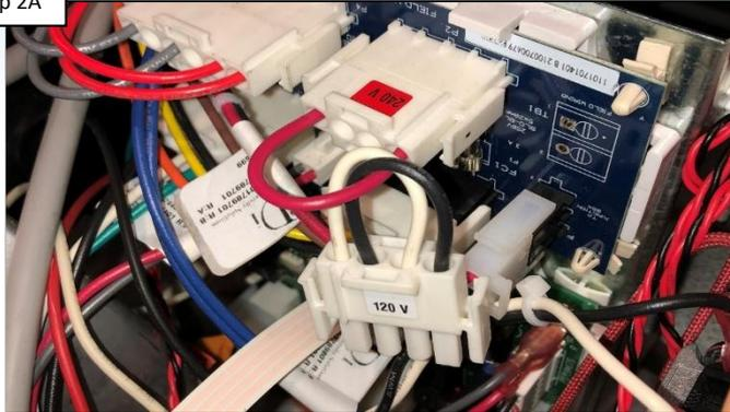
IF voltage selector plug matches voltage, go to step 2B. IF not, power down, replace FC1 & FC2 fuses, & switch plug to proper voltage.
