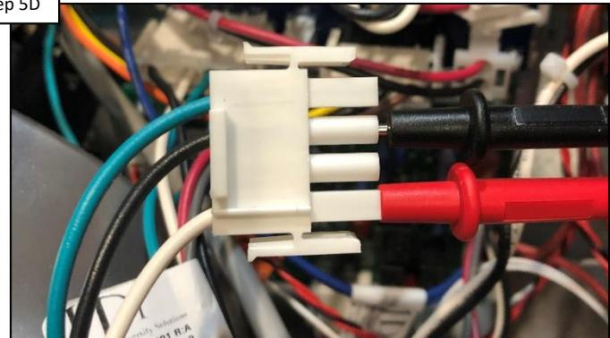
Disconnect the E10 connector from ICB. Verify 110-125VAC between 1-3 (white & black). IF present, replace ICB. IF NOT, replace wire harness (pg. 25).
