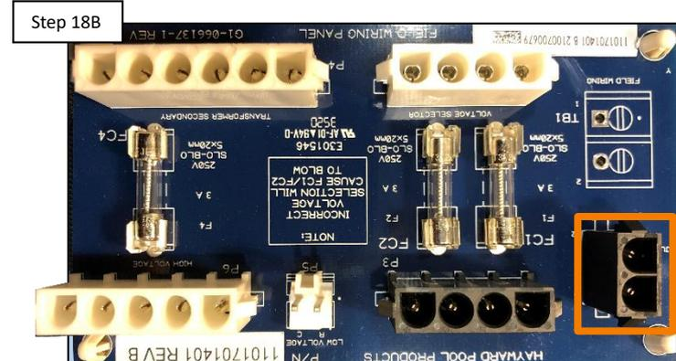
Unplug the wire harness from the P1 terminal and test voltage on the harness (115VAC or 230VAC). IF incoming voltage is out of range (+/-10%), repair incoming voltage. Otherwise, replace the ICB (pg. 25).
