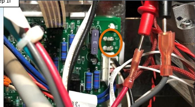
Disconnect and test the red and grey wires from the ICB. IF 22-28VAC is present go to step 1J. IF NOT, replace wire harness (pg. 25).
