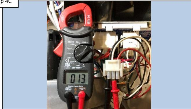
Measure for 13-18 ohms across the black and white (red wire not used) terminal wires. IF out-of-range, replace blower (pg. 25). IF correct, contact technical support (908)355-7995.
