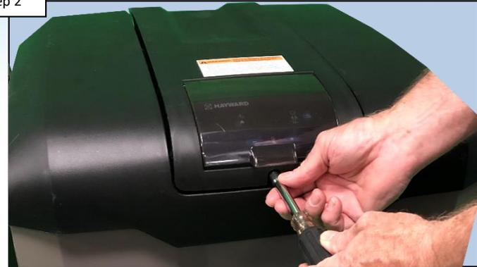
Using a 5/16 nut driver or #2 Phillips Head screwdriver, remove screw from below display.
