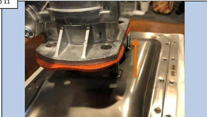
Lift straight up to remove blower assembly from the burner. Gently lay the blower aside.
