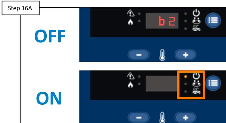
Power cycle heater, in an attempt to clear the “b2” code. IF power cycling clears to the “b2” message and the heater fires, drop the temperature to suspend heating. IF “b2” reappears, go to step 16B.
