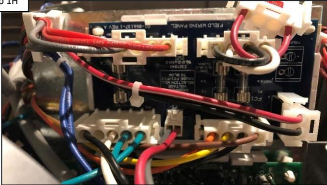
Inspect ICB wiring, ensuring all plugs are securely fastened. IF wiring is OK go to Step 1I. IF NOT, secure wiring/plugs then retest.
