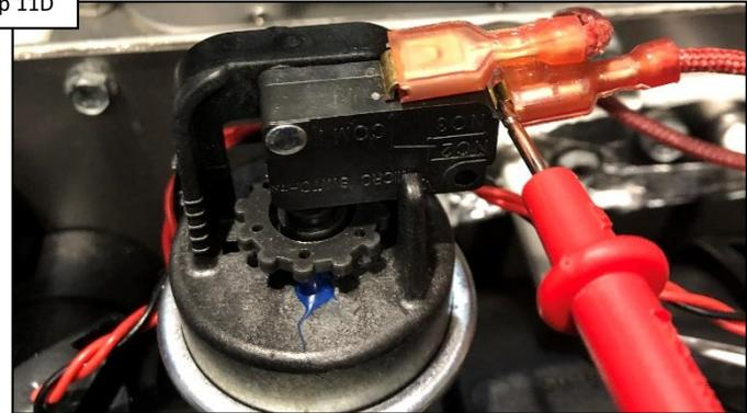
Test for 24V AC on the opposite terminal on the water pressure switch. IF no voltage, replace water pressure switch ([pg. 25](#)). IF OK, go to Step 11E.
