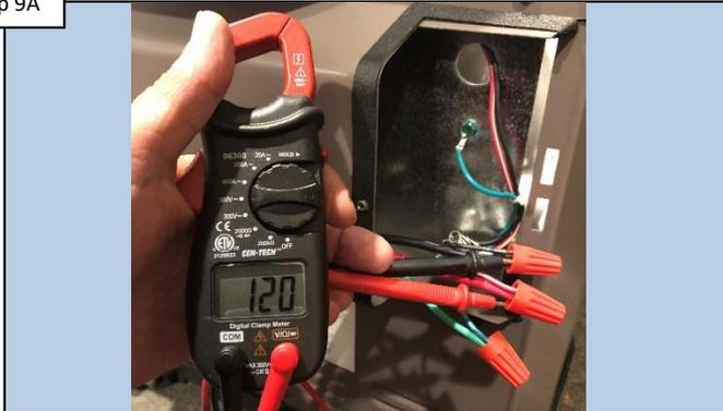
Ensure voltage is within 10% + or – of required voltage. IF voltage is correct, go to step 9B. IF NOT, then the problem is related to source power and must be corrected before error will clear.
