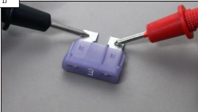
On the ICB, locate and test the 3A fuse for continuity. IF fuse is blown, replace it and go to Page 30. IF Ok, go to step 1K.
