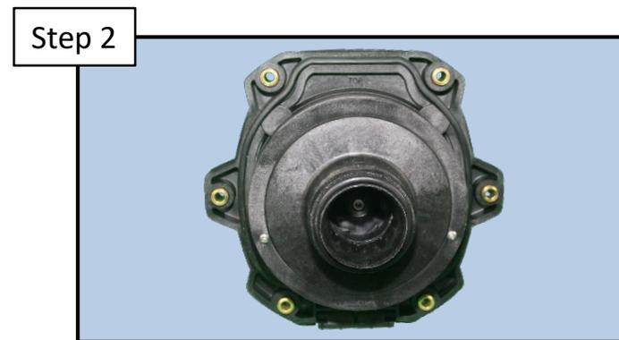
Turn power off for 30 seconds. If motor still will not start replace the power end. Check [pages 38-47](#) of this manual for parts list.
