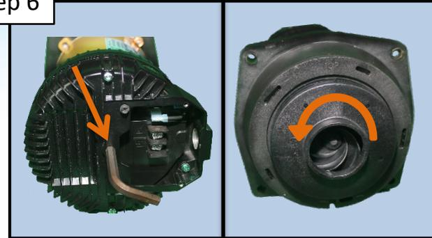
Slide a 5/16" Allen wrench fully into the shaft hold socket to secure the shaft so it does not spin. Rotate the impeller counter-clockwise to remove.
