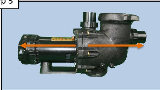
Pull the power end assembly away from the pump housing. This will provide you with access to the diffuser, impeller, impeller ring, and shaft seal.
