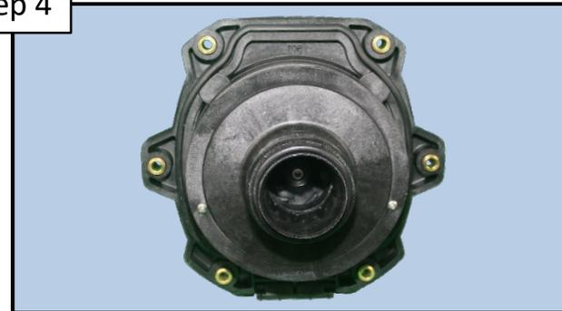
Power end must be replaced. Make certain the voltage jumper is correct prior to applying power to the pump. ([pages 38-47](#))
