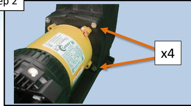
Remove the four (4) 9/16" bolts from the seal plate.
