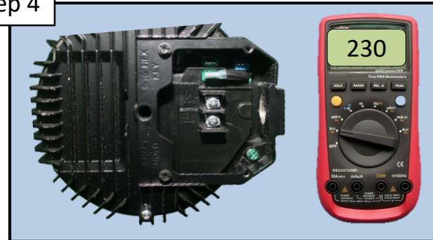
Verify input **AC** voltage at the motor is within 10% of applied voltage. If not within 10%, have the voltage corrected. If within 10%, replace the pump power end. ([pages 38-47](#))
