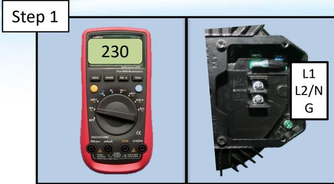
Verify input **AC** voltage at motor is within 10% of applied voltage. If not within 10%, correct voltage. If within 10%, go to step 2.
