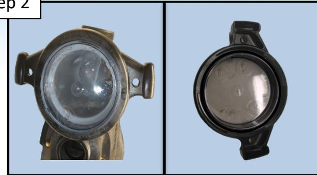
Make certain pump lid is installed correctly. Check O-ring inside the pump lid for any debris or signs of damage. Proceed to step 3.
