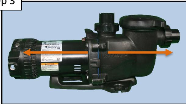
Pull the power end assembly away from the pump housing. This will provide you with the ability to access the diffuser, the impeller, and the shaft seal.
