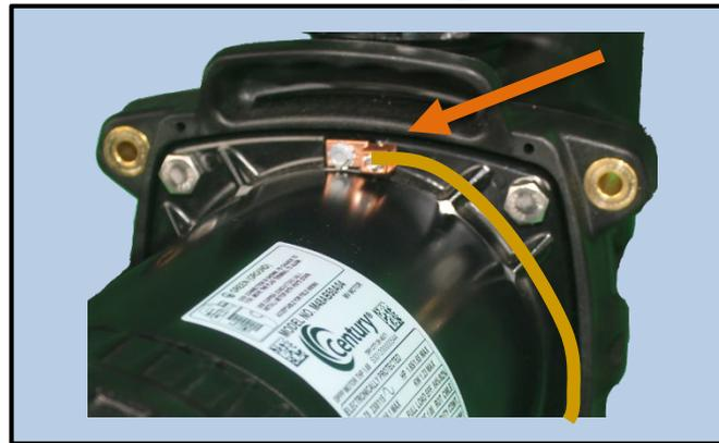
Secure #8awg bonding wire to the bonding lug as required by the National Electrical Code.
