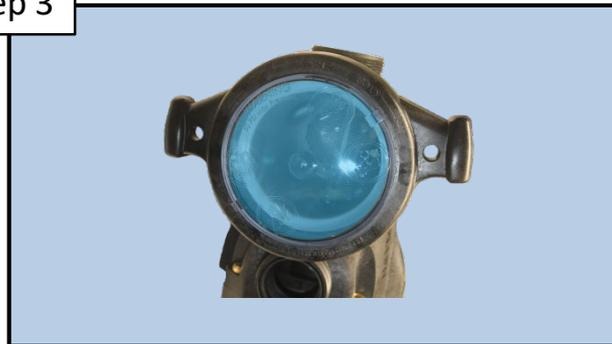
Clear any debris from basket and fill completely with water. Secure lid to housing and attempt to prime pump. If pump does not prime proceed to step 4.
