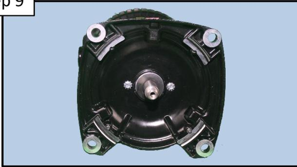
If replacing the XE power end, it is important to use the correct power end for the pump model. See parts breakdown on [pages 38-47](#).
