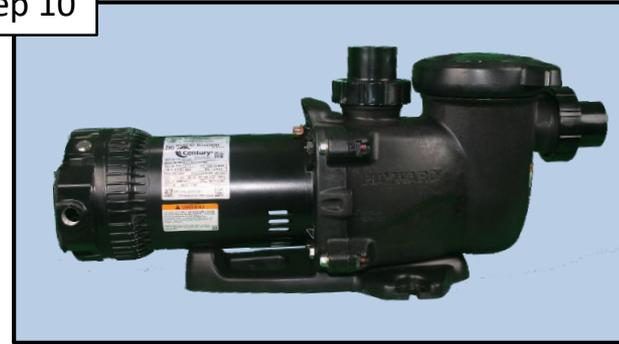
Reverse steps 1-8 to re-assemble pump. Be sure to configure the wiring properly for input voltage.
