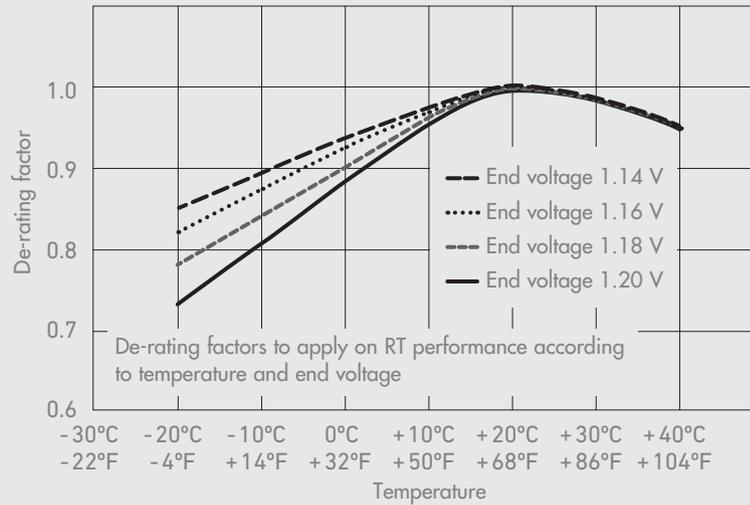
**Figure 2. Temperature de-rating: special electrolyte for operating temperatures down to -40°C (-40°F).**
