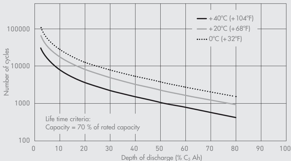
**Figure 5. Sunica.plus cycling to IEC Standard 61427-1**
