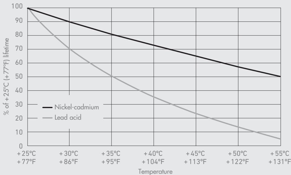
In general terms for every +10°C (+18°F) increase above +25°C (+77°F), the calendar life of the Sunica.plus is reduced by 20%. The lead acid battery is reduced by 50% in the same case.
