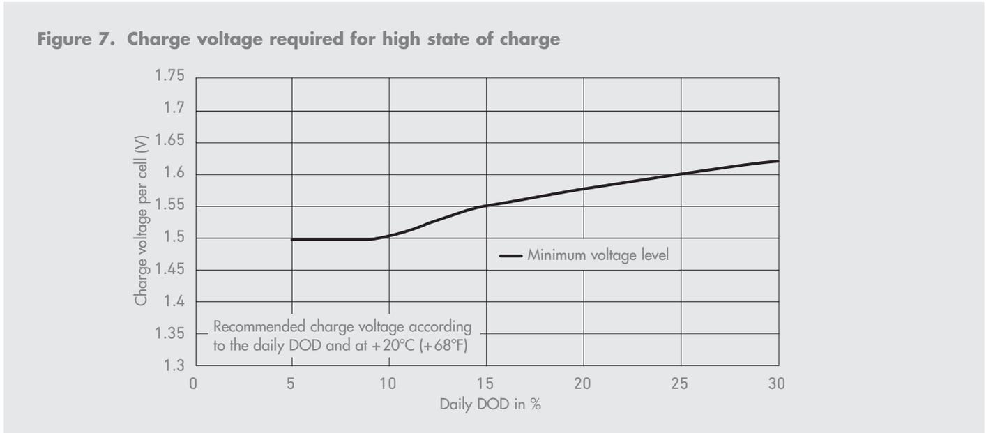
When cycling with this recommended charge voltage, the Sunica.plus will stabilize at greater than 95 % state of charge. The solar panels should be sized to provide a minimum needed energy to maintain this high state of charge. Values for the minimum needed charge energy is provided in the Saft sizing outputs.
