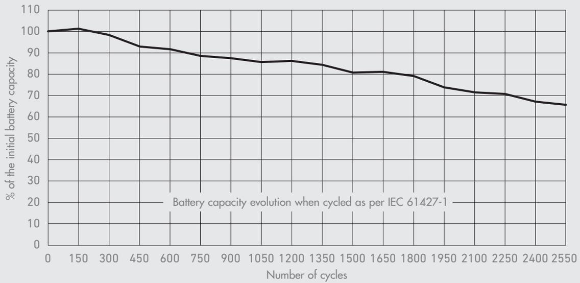
The Sunica.plus delivered 1800 cycles according to IEC 61427-1 (see Figure 5). The test results demonstrate its superior cycling ability after being subjected to continuous cycling at a partial state of charge (low and high) and at a fixed +40°C (+104°F).
