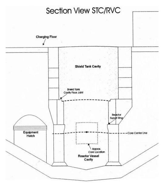
Figure A-1 Cross Section of Yankee Rowe Containment Building
