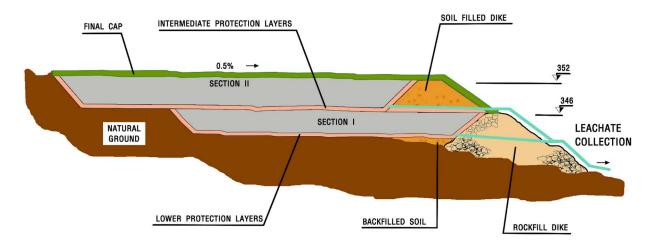
Figure 5-5 Longitudinal View of Trench 29 [11]
