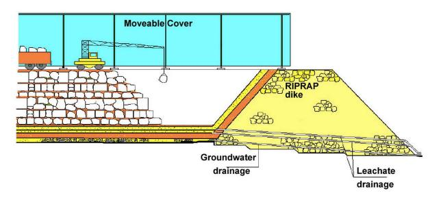
Figure 5-6 Side view of a Section 1 of a VLLW Disposal Trench at El Cabril [10]
