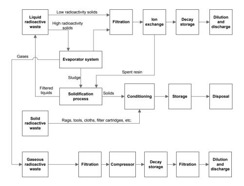
FIG. I–1. Generic (major processes) flow chart of the management of radioactive waste in a nuclear power plant or research reactor. Figure adapted from NUREG/CR1759<sup>1</sup>.
