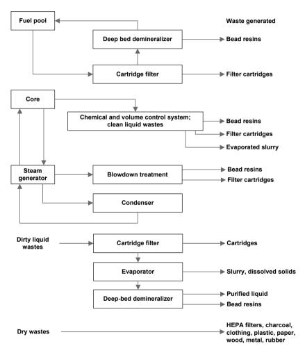
FIG. II–1. Example of a flow chart of the management of radioactive waste in a pressurized water reactor (partial flow condensate polishing). Figure adapted from NUREG/CR1759<sup>1</sup>.
