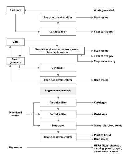
FIG. III–1. Example of a flow chart of the management of radioactive waste in a pressurized water reactor (full flow condensate polishing). Figure adapted from NUREG/CR1759<sup>1</sup>.
