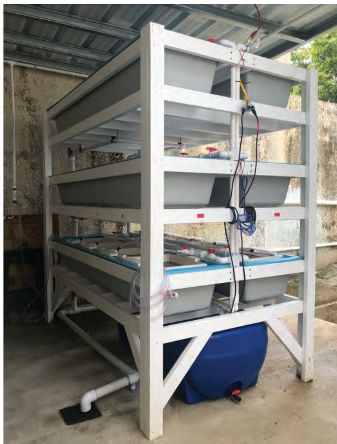
FIGURE 5. Nursery recirculating aquaculture system used for the study and designed for growing queen conch juveniles (Photo: Chaler Dones-Ortiz).
