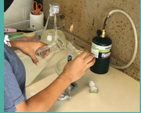
3.b Small flask on the right has inoculum. Large flask small on the left is recipient.
