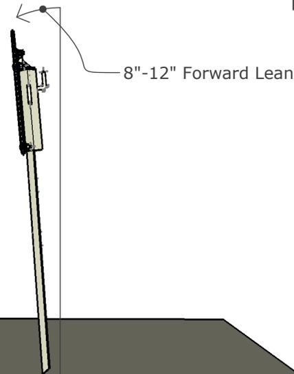
Lean the target towards the shooting position ~8"-12". This does not need to be exact and the target will function at a straight vertical position. The forward lean makes shooting the target safer by directing fragments downward and assists in the function of the HFR Flipper if applicable.
